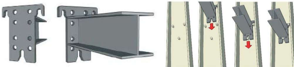
Figure 14: Slotted connection assembled by displacement (Bijlaard, Girao Coelho, & Magalhaes, 2009)
