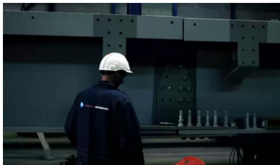
Figure 10: Beam splice used in Janson modular bridge (left) (Janson Bridging) and cross-section from the brochure of the corresponding type (right) which has been used to determine cross-section properties (Janson Bridging , 2011)
