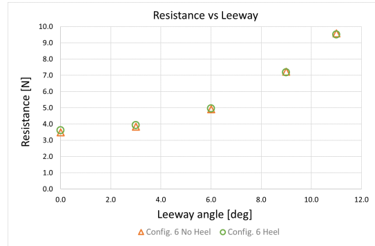
Figure 5.7: Resistance versus leeway angle of configuration 6 upright and heeled.
