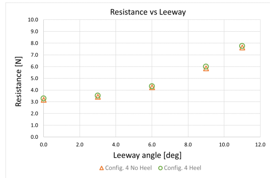
Figure 5.5: Resistance versus leeway angle of configuration 4 upright and heeled.
