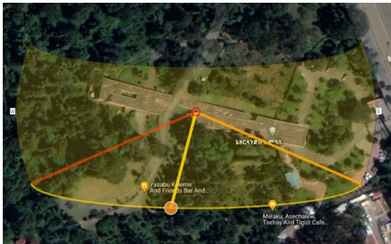
Figure 23: Sunpath on the location at 25 December, at 13:00. From 'Computation path for the sun for Addis Ababa,' by Suncalc, n.d.( https://www.suncalc.org/#/9.0194,38.7152,19/2023.12.25/13:00/1/1 ).
