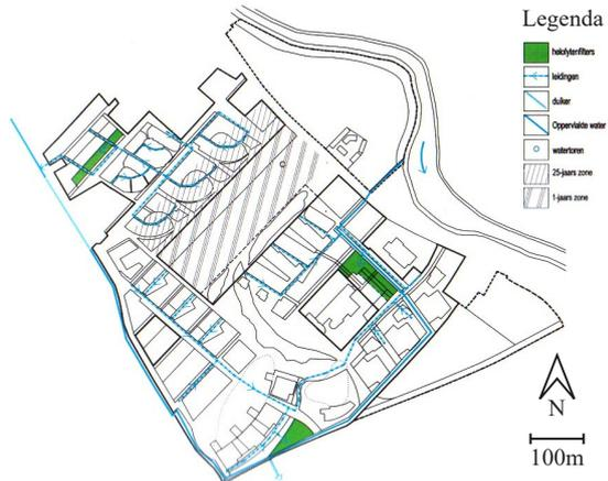
Figure 10. The greywater system of Lanxmeer with the helophyte filters (EVA-Lanxmeer, n.d.)
