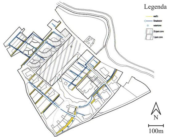
Figure 12. The street rainwater system in Lanxmeer with the wadis (EVA-Lanxmeer, n.d.)
