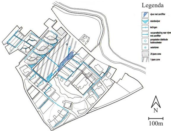
Figure 11. The roof rainwater system in Lanxmeer with the retention ponds (EVA-Lanxmeer, n.d.)
