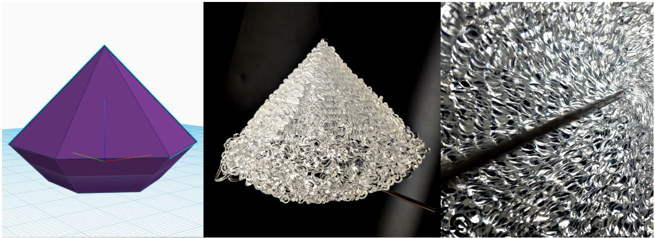
Figure 5: An upside-down diamond shape (created in Tinkercad) fabricated with the dribbled rope coiling technique where the height, speed and flow are interactively controlled. An internal detail of the texturing created is seen in the right panel, far different from traditional 3D printing.
