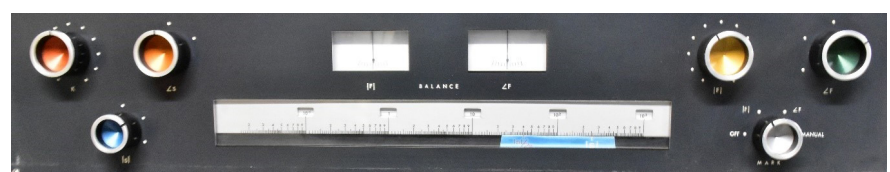
Figure 6. The null-meters, the s-scale and various controls
