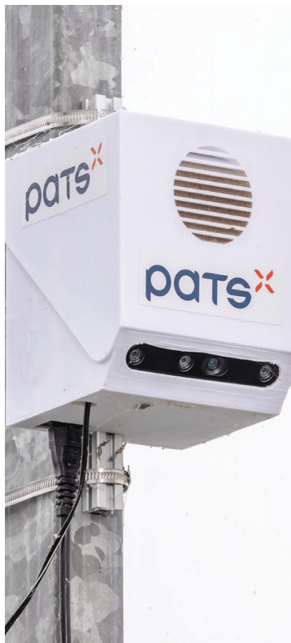
Figure 2. Stationary camera that detects and tracks moths inside the greenhouse
