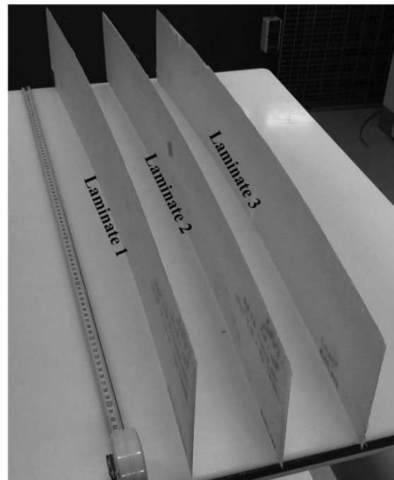
Figure 3. Experimental warpage for the three manufactured laminates.
