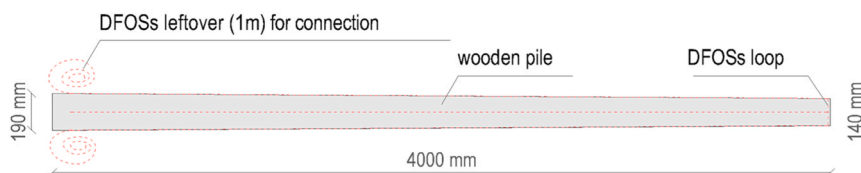
Fig. 7. DFOS set-up over the pile tip (V_V).
