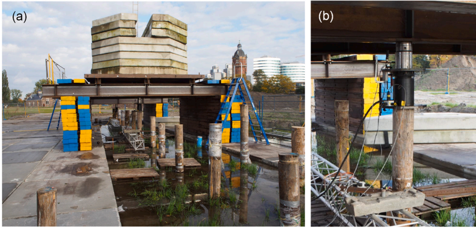
Fig. 3. (a) In-situ loading set-up applied to a wooden foundation pile in Overamstel (Amsterdam, NL); (b) LVDTs applied to the pile head to monitor the displacement during loading.
