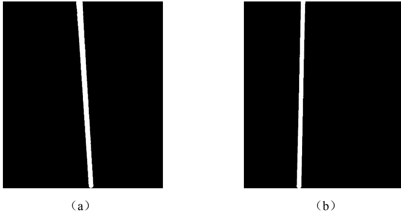
Fig.10. Threshold segmentation image: (a) VMI tear image; (b) VFI wear image
