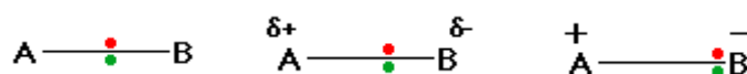
Figure 4.5. How the electrons are shared between the atoms depends on the electronegativity. If the electronegativity of two atoms is the same, a covalent bond arises (left), if one atom has a slightly higher electronegativity that atom pulls the electrons slightly towards it, resulting in a polar bond (middle) and if the electronegativities differ significantly, this can result in the electrons being pulled towards one atom to such an extent that the other atom ionizes and an ionic bond arises (right).
