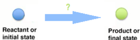
Figure G.2. The objective of NEB is to find the minimum energy path from an initial to a final state. 68
