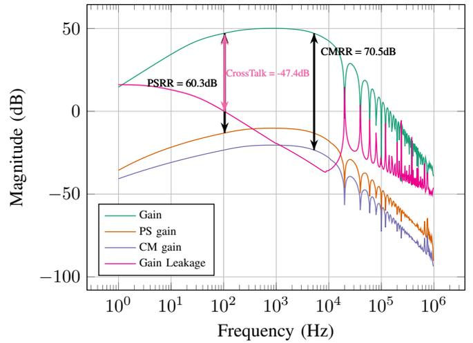
Fig. 8: Post-layout simulation results for the gain, CM gain, PS gain, and gain leakage with annotated CMRR, PSRR, and crosstalk.
