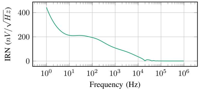
Fig. 9: Input referred noise voltage (IRN) power spectral density.
