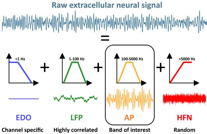
Fig. 2: Raw extracellular neural signal components.
