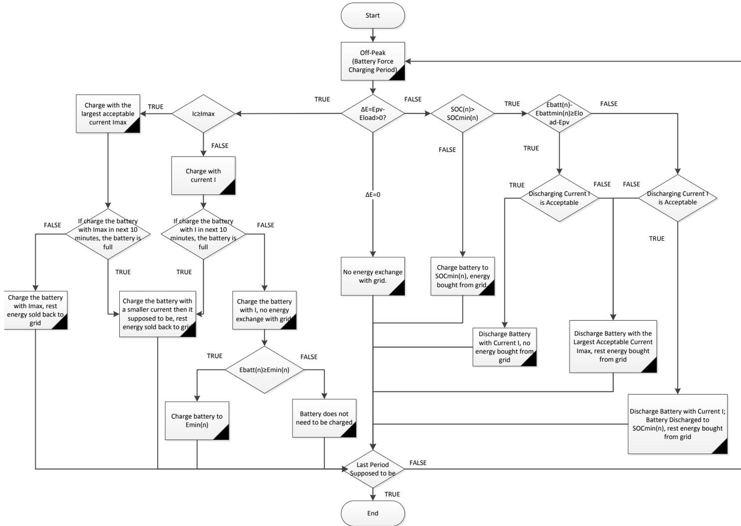
Figure 3.6: Power Flow for PMM2 and PMM3 During the Battery Forced Charging Period
