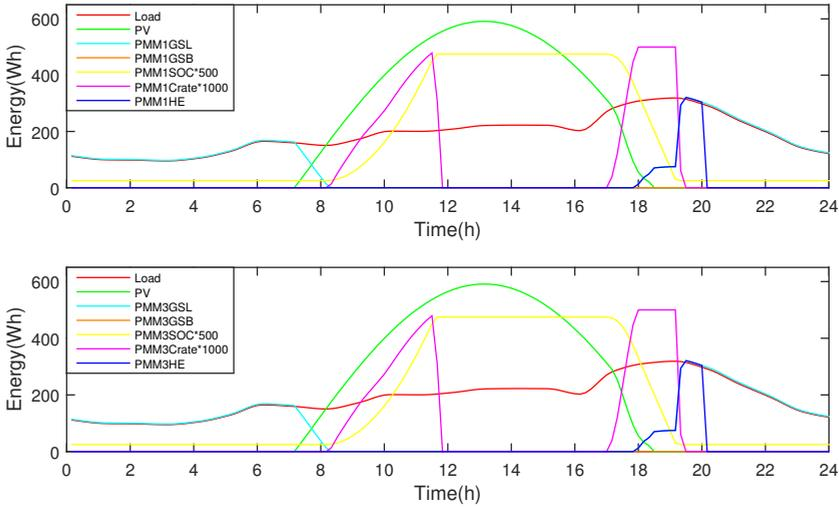
Figure 3.35: PMM1 and PMM3 Energy Flow Comparison (California-1 Battery)
