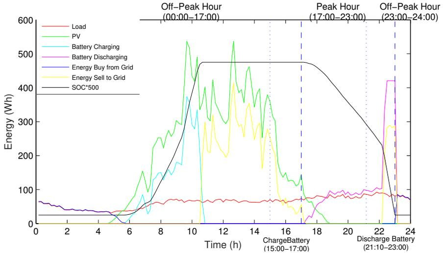
Figure 3.10: Power Flow of Power Management Three (April 28th)
