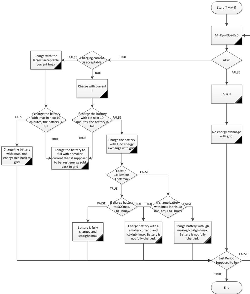
Figure 3.12: Power Flow for Power Management Method ( $P_{PV} \geq P_{load}$ )
