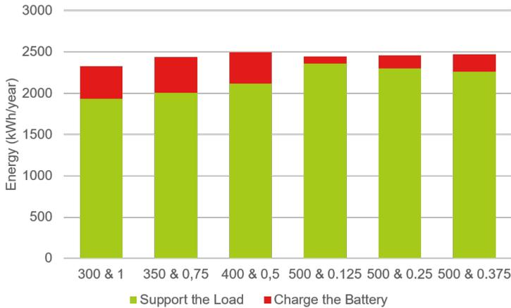
Figure 3.24: The Total Energy Bought from the Grid with Different Reference Value for Peak-Shaving
