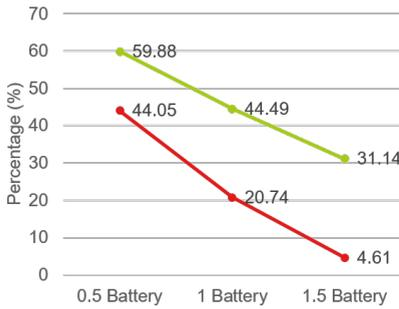
Figure 3.25: Peak-Hour Energy Consumption-Total Energy Consumption Ratio (PMM1 and PMM2)
