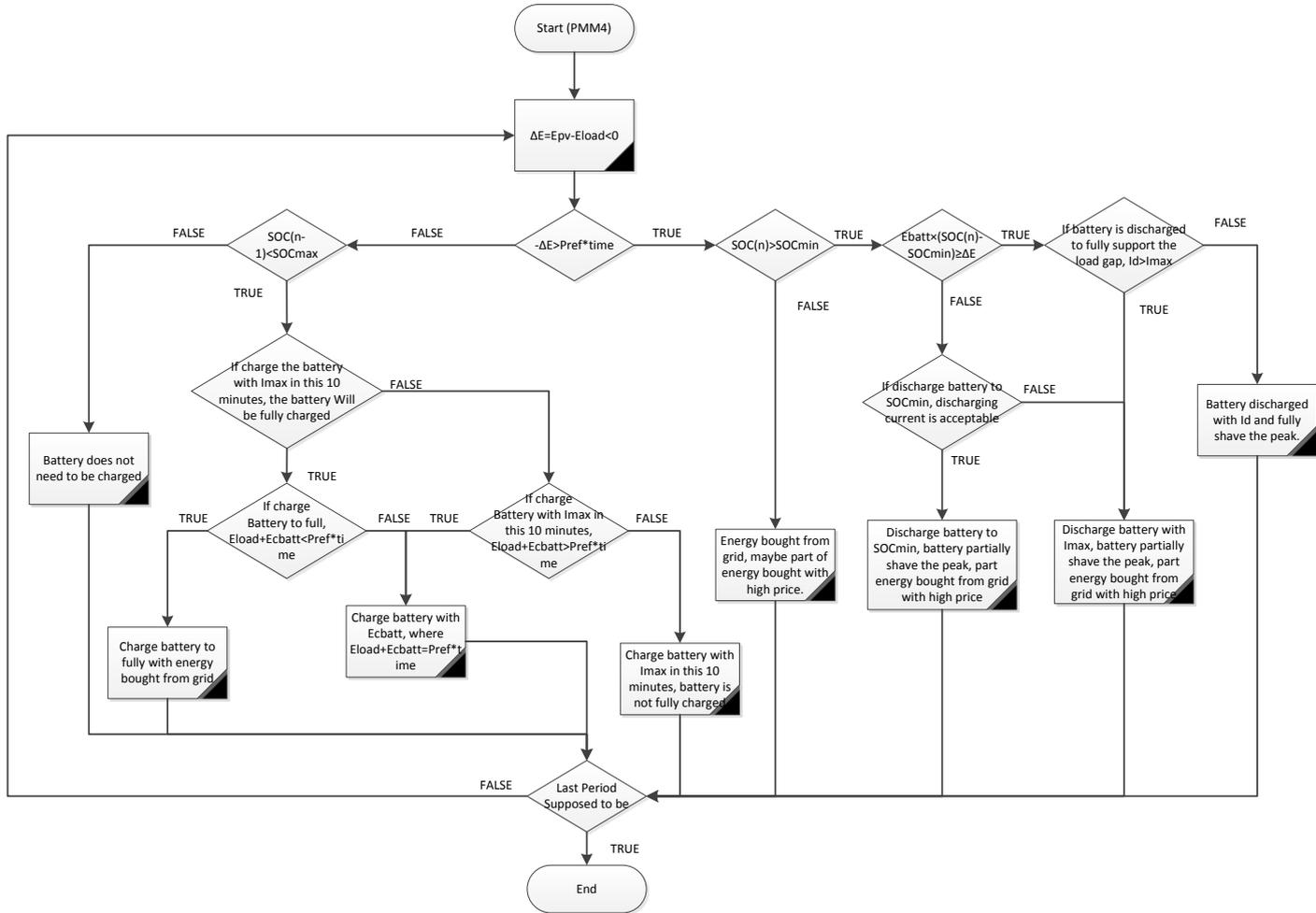
Figure 3.13: Power Flow for Power Management Method ( $P_{PV} < P_{load}$ )
