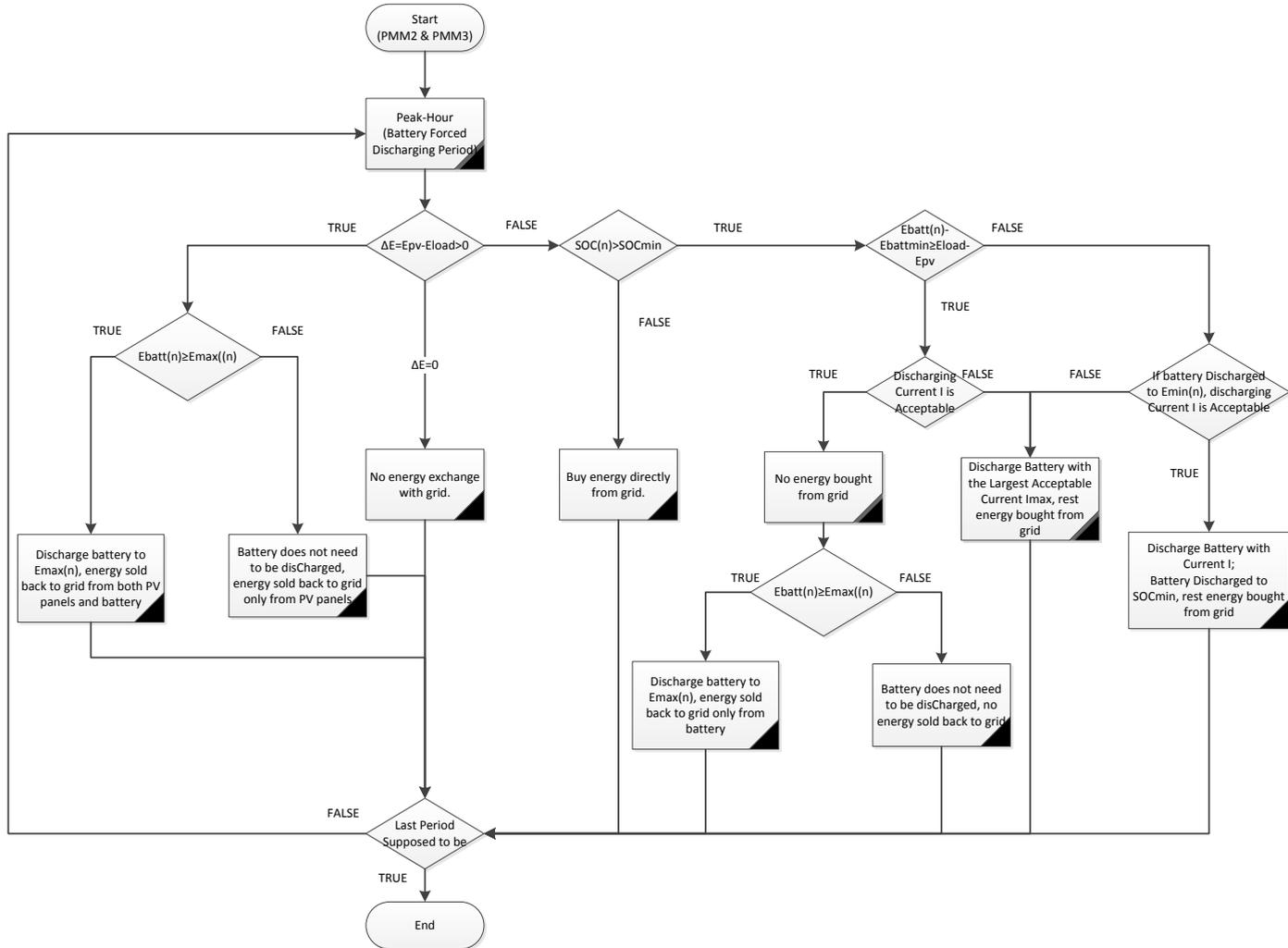
Figure 3.8: Power Flow for PMM2 and PMM3 During Battery Forced Discharging Period
