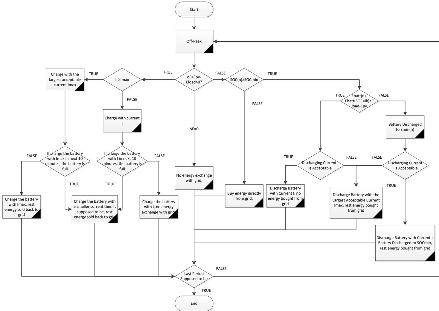
Figure 3.5: Power Flow for PMM2 and PMM3 During Off-Peak-Hour (Before the Battery Forced Charging Period Starts)
