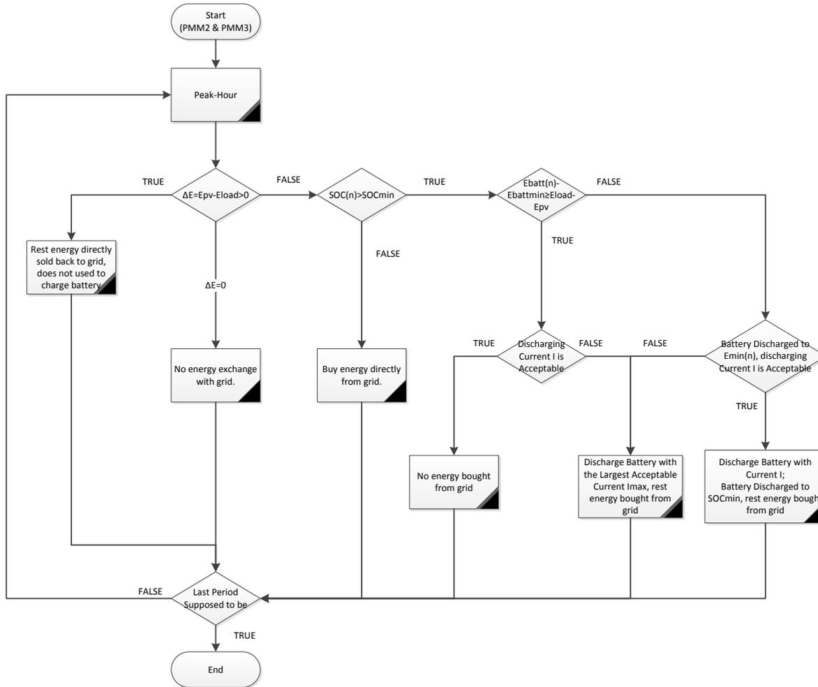
Figure 3.7: Power Flow for PMM2 and PMM3 During Peak-Hour (Before the Battery Forced Discharging Period Starts)
