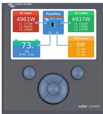
**Color Control Panel, showing a PV application**
