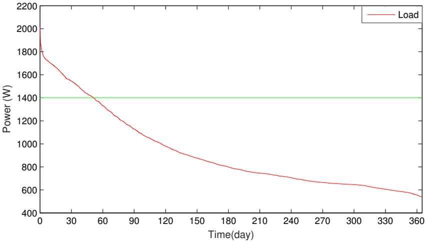
Figure 3.16: Load Profile in Descending Order (California)
