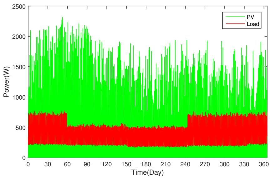
Figure 2.13: PV Generation Profile and Load Profile for Costa Rica
