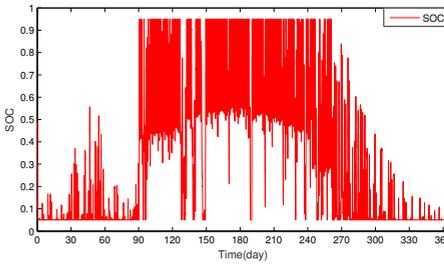
Figure 2.15: SOC for 1 Battery
