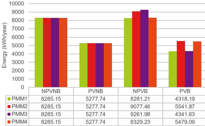
Figure 3.38: Comparison of Energy Bought from Grid Between NPVNB, PVNB, NPVB and PVB (California)
