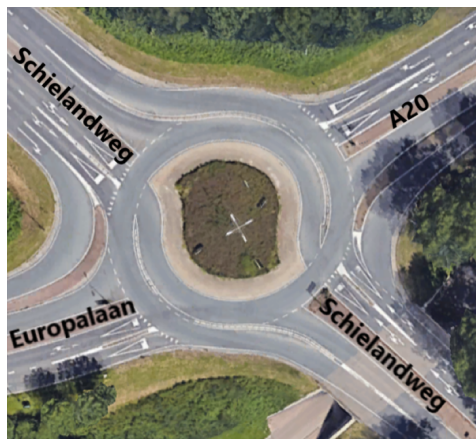
Figure 3.1: Aerial overview of a turbo-roundabout in Nieuwerkerk aan den IJssel, the Netherlands. The street names are depicted in black.
