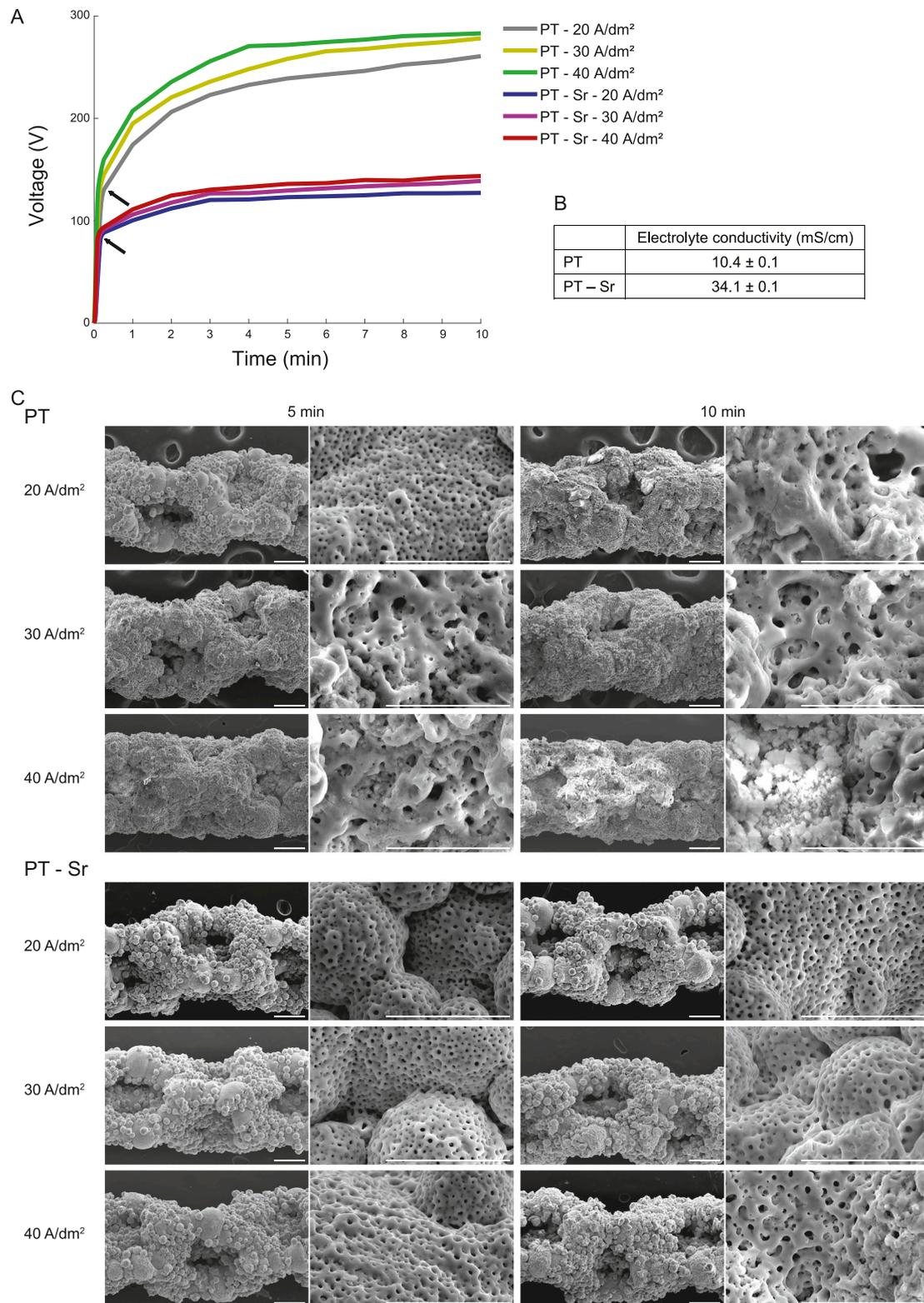
**Fig. 1.** (A) The V-t transients registered during the PEO processing of AM Ti-6Al-4 V implants. Arrows indicate dielectric breakdown. (B) The electrolyte conductivity of PT and PT - Sr electrolytes ( $n = 3$ ). (C) The SEM images showing the surface morphology of the implants after PEO biofunctionalization. Scale bars are 200  $\mu\text{m}$  (low magnifications) and 40  $\mu\text{m}$  (high magnifications).
