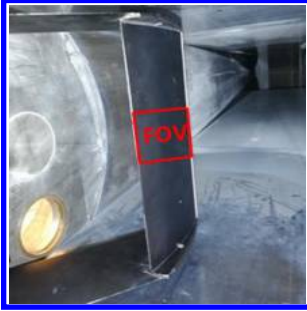
Fig. 4 Second PIV experiment: “vertical” airfoil mounted in the wind tunnel with relative FOV (left) and sketch of the airfoil with the plane of measurement in green and \lambda -shock structure in blue (right).
