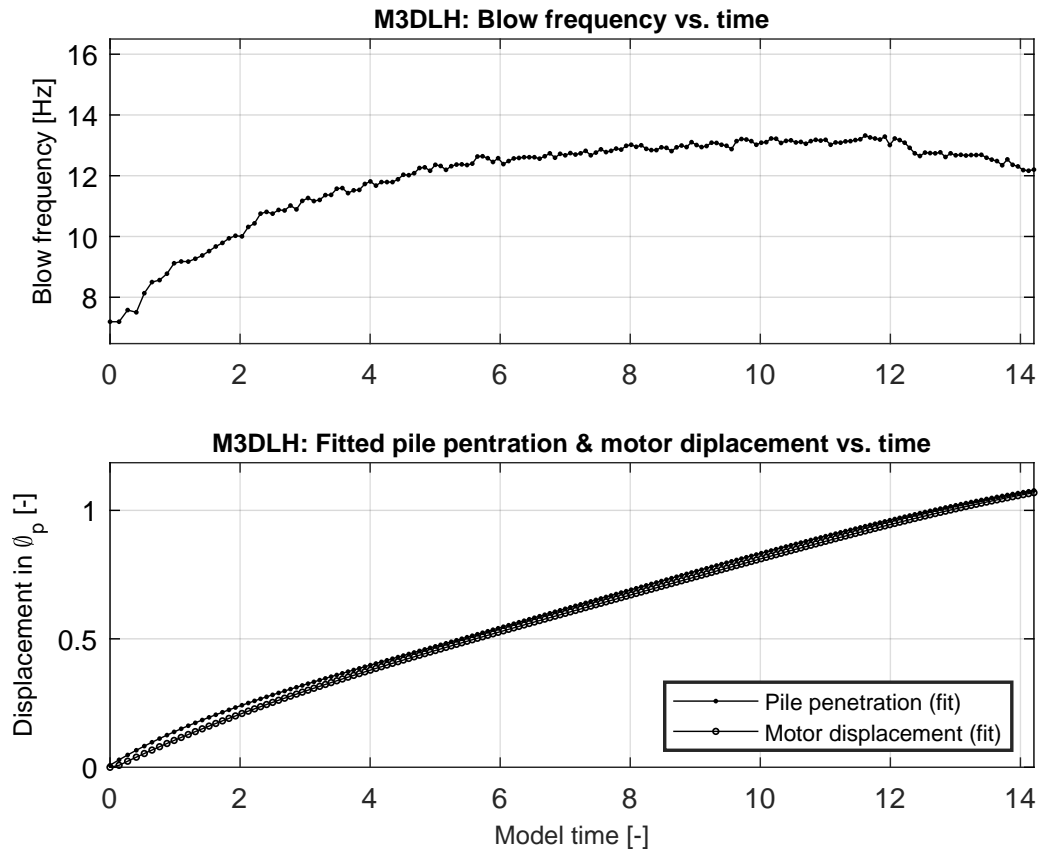
Figure C.68: (TOP) Driving frequency evaluated per blow as a function of model time for test M3DLH. As the frequency is inferred based on time intervals between triggers of the load cell, the frequency for the first blow cannot be determined. Instead, it is equaled to the frequency estimate for the second blow. (BOTTOM) Fitted expressions for PP and MD, evaluated per blow as a function of model time for M3DLH
