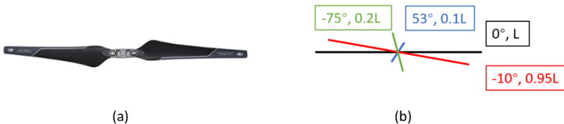
Figure 3.3: (a) Blade of DJI 2170 propeller (b) Multi-wire model of propeller blade
