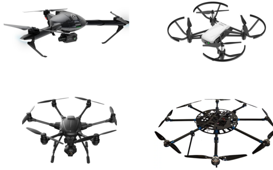
Figure 3.1: Different types of drones (a) tricopter, (b) quadcopter, (c) hexacopter, and (d) octocopter
