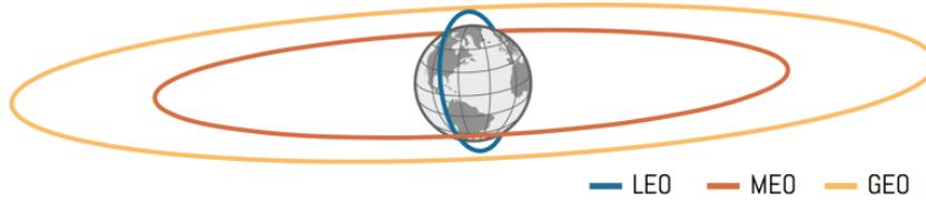
Figure 2.2: The figure shows the characterization of three orbits namely Low-Earth Orbit (LEO), Medium-Earth Orbit (MEO) and Geosynchronous Orbit (GEO) as given by [11].
