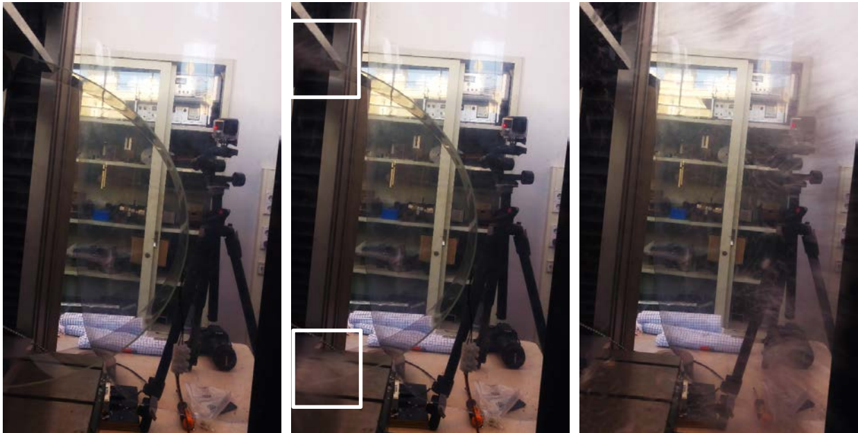
Fig. 15 Frames of the collapse, highlighting the frame the glass breaks at the slits (centre picture) and the following frame (right picture)
