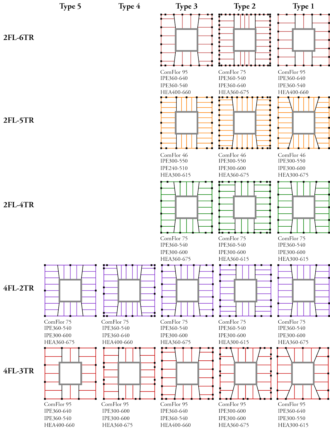
Figure B.11: Overview of the composite floor configurations for the 200-meter diagrid models. The castellated beams are indicated as IPE300-600 where IPE300 is the original profile and 600 is the height of the castellated beam.
