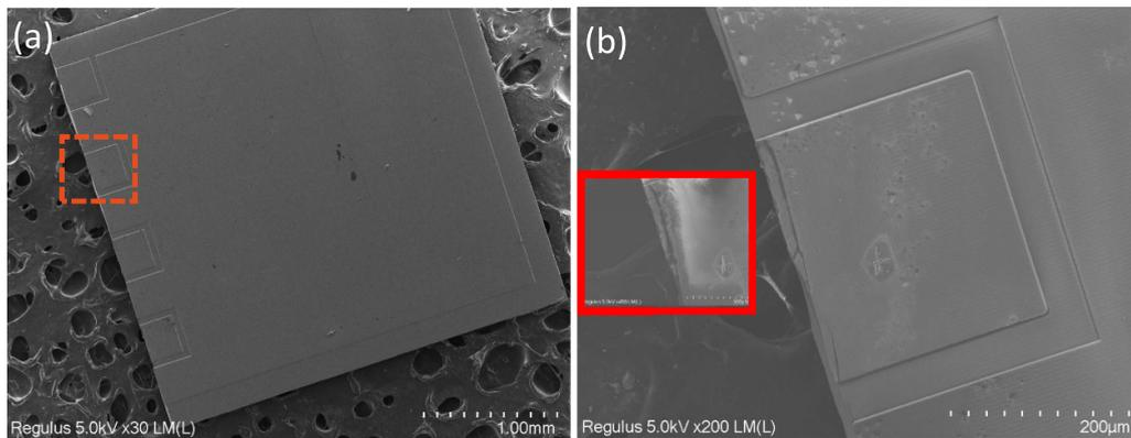
**Figure 12.** (a) SEM analysis of thin meander chip shows crack propagation across metal absent isolated 50 µm gap. (b) Close-up image showing fracture origin and propagation across vertical trenches underneath.
