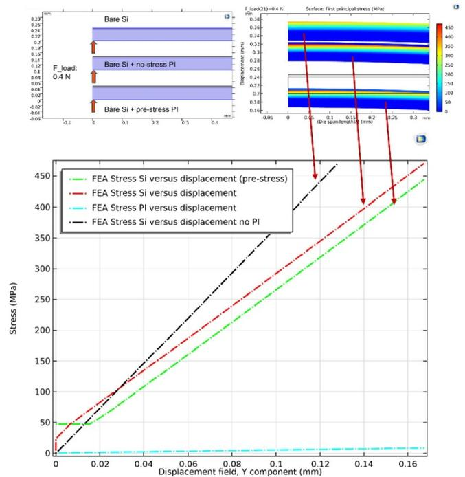
**Figure 16.** Different models exhibiting stress levels are required for die fracture. The sample with pre-stressed PI film shows the lowest stress.
