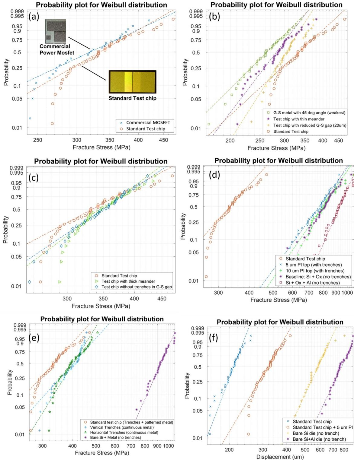
**Figure 10.** Probability plot for Weibull distribution (a) comparing commercial die with fabricated standard test chip. (b) Die designs with weaker strength to standard die (c) robust die designs, (d) PI influence on die robustness, (e) trench orientation influence on die strength. (f) Die bending displacement for different dietop samples.
