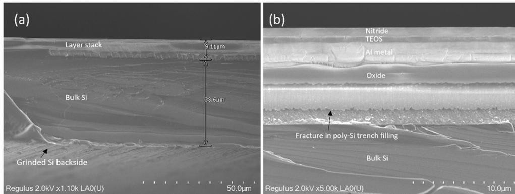
**Figure 9.** (a) SEM analysis of fractured die indicating Bulk Si and layer silicon of 48  $\mu\text{m}$  thick die, (b) close-up indicating fracture propagation across polysilicon-filled trenches.
