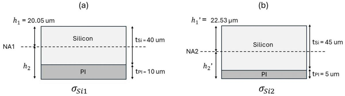
**Figure 8.** Cross-section diagram of the two 50 μm composite beams with different thicknesses of silicon and polyimide films, (a) indicates the overall beam neutral axis with deposition of 10 μm PI versus (b) a shift in the neutral axis with 5 μm PI deposition.
