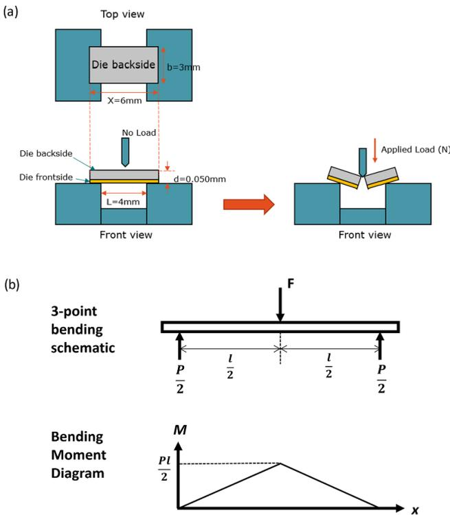
**Figure 7.** (a) Top and front view of die loading setup where  $l$  is span length,  $x$ ,  $b$  and  $d$  are sample length, width and thickness respectively, (b) schematic of the TPB test setup with bending moment distribution where  $F$  is applied load,  $l$  is loading span.
