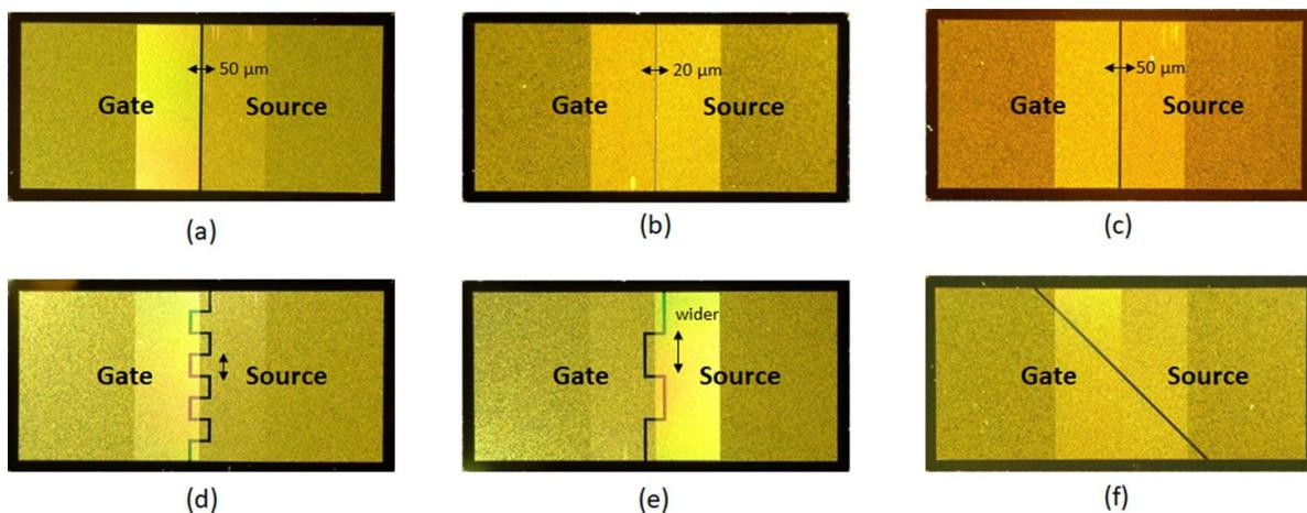
**Figure 4.** Die topside view showing (a) reference die with gate-source separation of 50 µm (b) gap reduced to 20 µm (c) die topside covered with PI (d) thinner meander pattern (e) meander pattern with wider metal area (f) 45° angled pattern separation.
