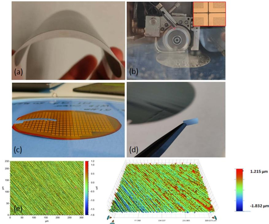
**Figure 5.** (a) High flexibility of ultrathin Si wafer, (b) dicing process and dicing kerf across dicing marker, (c) diced wafer on Adwill D-175 UV tape, (d) tweezer assisted manual die pickup. (e) 3D plot for die backside roughness.
