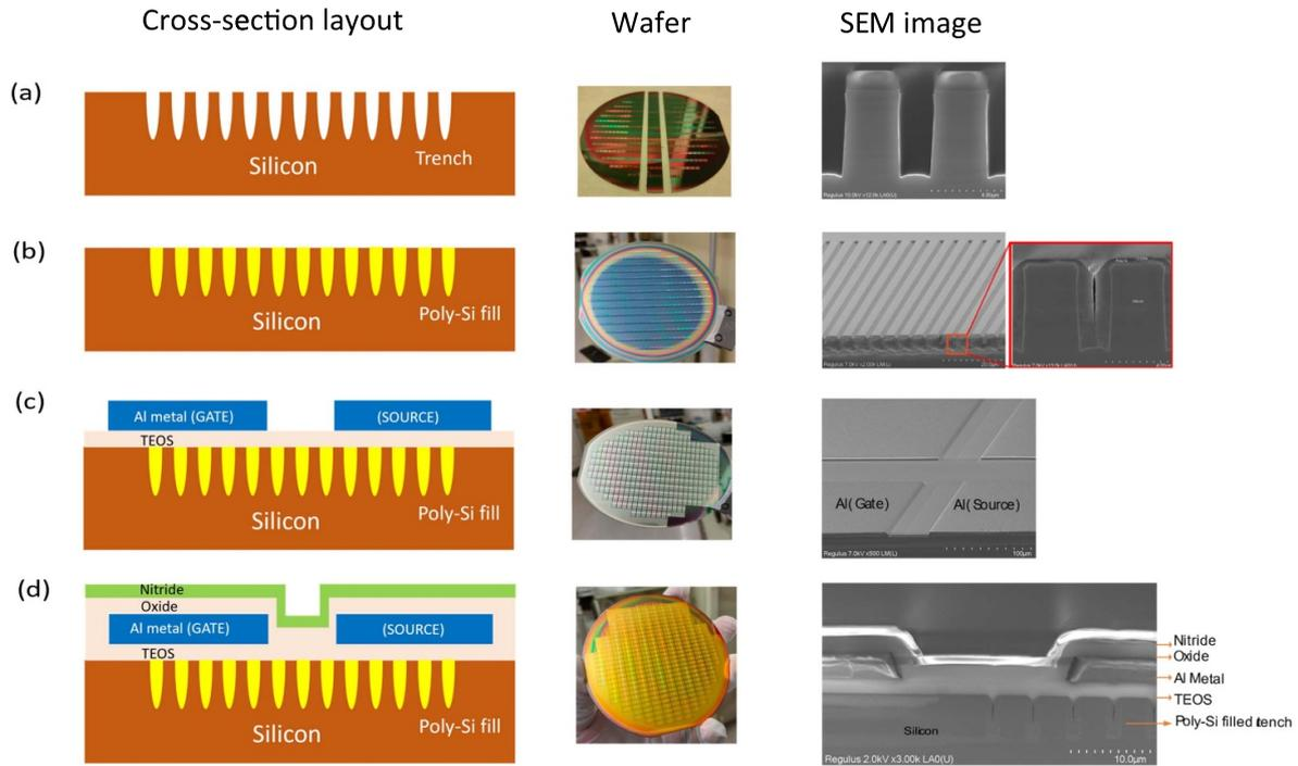
**Figure 1.** Process flow for dummy power MOSFET device fabrication. Processed wafers and cross-sections are shown. (a) Trench formation in silicon; (b) trenches are filled with poly-Si and etched back to remove excessive poly-Si from wafer top; (c) an insulating layer of TEOS, followed by pure Al is sputtered on top and patterned to form gate-source regions. (d) The metal top is covered with passivation films of oxide and nitride.
