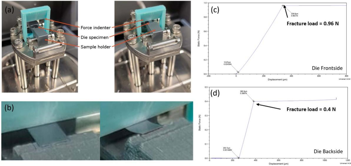
**Figure 6.** (a) DMA test setup with 3D printed indenter for three-point bend test. (b) Deflection as shown by die before and after applied load. (c) Load-deflection curve for bare Si frontside. (d) Load-deflection curve for bare Si backside.
