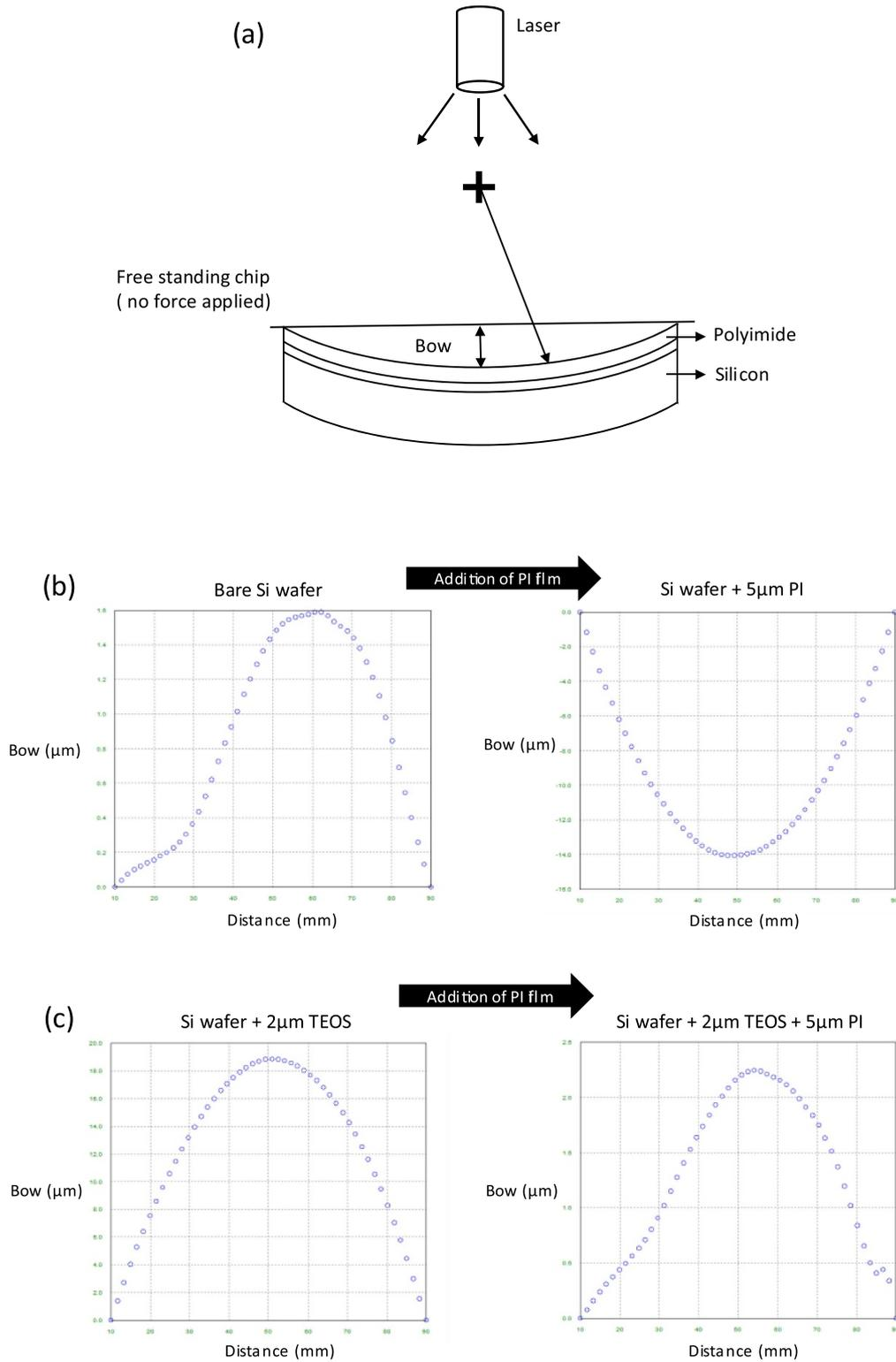
**Figure 15.** (a) Bow and radius of a warped Si sample with PI film as measured by Flexus thin film stress measurement tool; (b) Before and after effect of adding PI film to Si wafer bow measurements; (c) (b) Before and after effect of adding PI film to Si wafer with TEOS coating. Residual stress in cured PI exhibits tensile stress.
