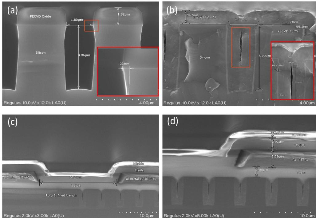
**Figure 3.** SEM image for wafer cross-section. (a) Hanging silicon groove in trench after dry etch step. (b) Trench void post poly-silicon filling. (c) Wafer cross-section showing MOSFET profile. (d) Close-up of the layer stack.
