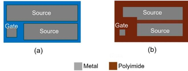
**Figure 14.** (a) Standard die layout; (b) proposed die layout with PI coating. The layout maximizes PI coverage with openings for gate-source interconnections. This design provides maximum robustness.
