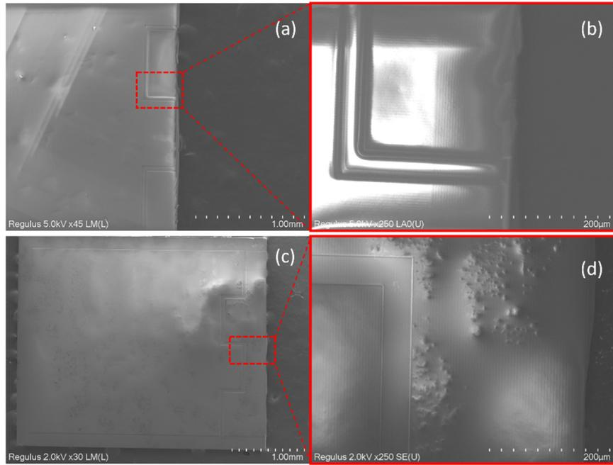
**Figure 11.** SEM image for die crack in thicker meander die. Two crack locations are identified (a) die fracture across metal absent insulation gap, (b) close-up image of crack origin in the vertical trench at source region. (c) Die fracture on metal-covered source region. (d) Close-up image of crack origin in vertical trench.
