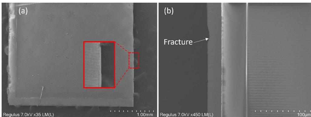
**Figure 13.** SEM fracture analysis of standard reference die vs die with modified trench layout, in modified samples, trenches were removed underneath metal isolation gap. (a) Die crack in middle across isolation gap in reference die, (b) crack across vertical trenches outside isolation gap in modified layout.
