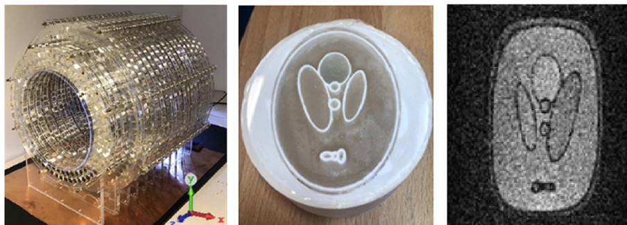
Fig. 2 (Left) A low-cost portable MRI at LUMC, (Middle) The 3D printed phantom (Shepp Logan) and (Right) The image of the 2D phantom acquired using the Low-Field MRI scanner on the left
