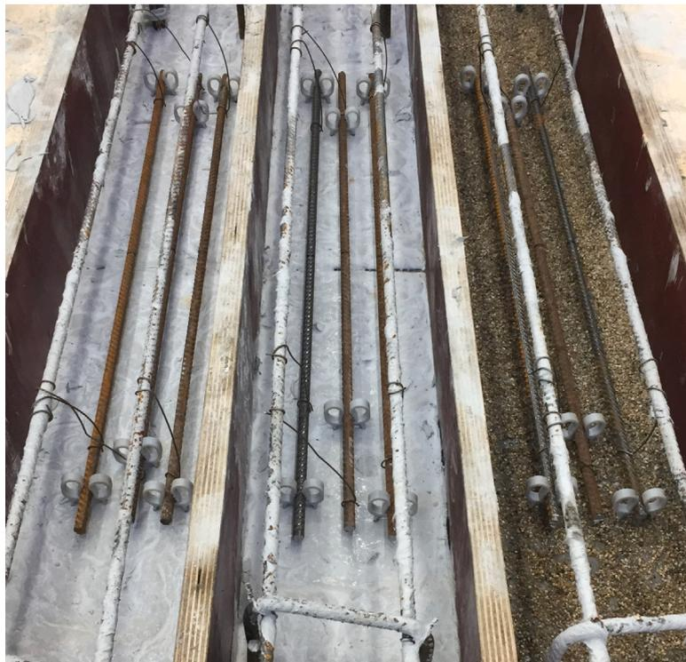
Fig. 3. Different types of interface preparation: smooth (“Reference” and “Curing”) and “Epoxy” sample with sand at the surface.
