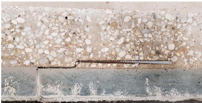
Fig. 11. Crack propagation in the Epoxy sample, within the beam, observed after cutting the sample in the middle.
