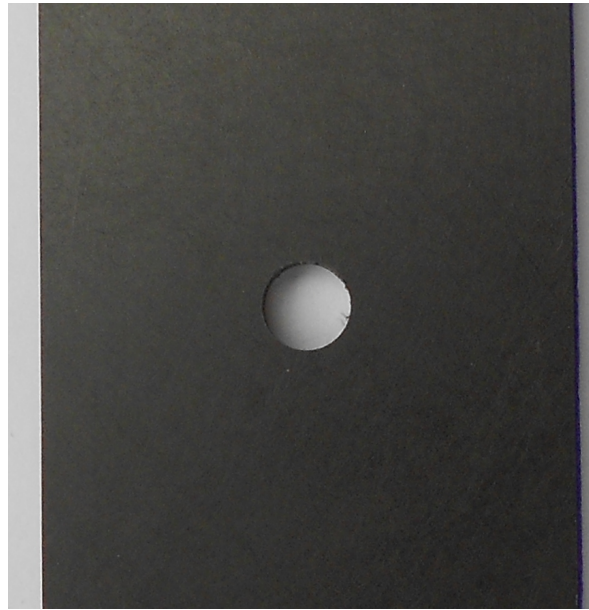
Figure 3.1: Milled hole in open-hole tension specimen
