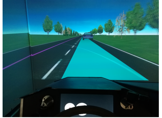
Fig. 4: Overview of designed visual systems from driver's perspective. Where purple line displays HCR (controllers trajectory), blue area the trend vector, and grey light line the yaw limits which indicate latest time moment of steering to prevent a collision. First visual system consists of HCR only, where second visual system contains all visuals.
