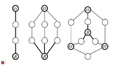
3 From left to right: graph representation of a particular serial robot, a parallel robot, and a parallel robot with a configurable platform. The actuated joints (in bold edges) are used to fully control the motion of each end-effector (EE) relatively to the base (B). base. High-speed pick-and-place robots and haptic interfaces are examples of applications which can benefit from this type of architecture. Figure 2 shows three PRCP examples with four, five and seven DoFs, respectively.
