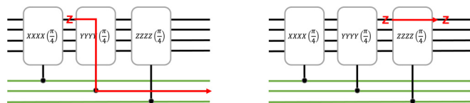
FIG. 11. Generalized Syndrome Measurement in analog with Shor-style syndrome measurement for [[4, 2, 2]] code. Ancilla qubits (green) are prepared in the GHZ state (|000\rangle + |111\rangle)/\sqrt{2} and each ancilla qubit controls a multi-qubit Pauli gate. An error occurred after the gates will either be detected (left) or commute with the following gates and will not propagate (right).
