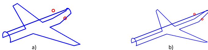
FIG. 8. Limit shadow-light and source position used in the predictions for (a) the F70 (b) the MD81.
