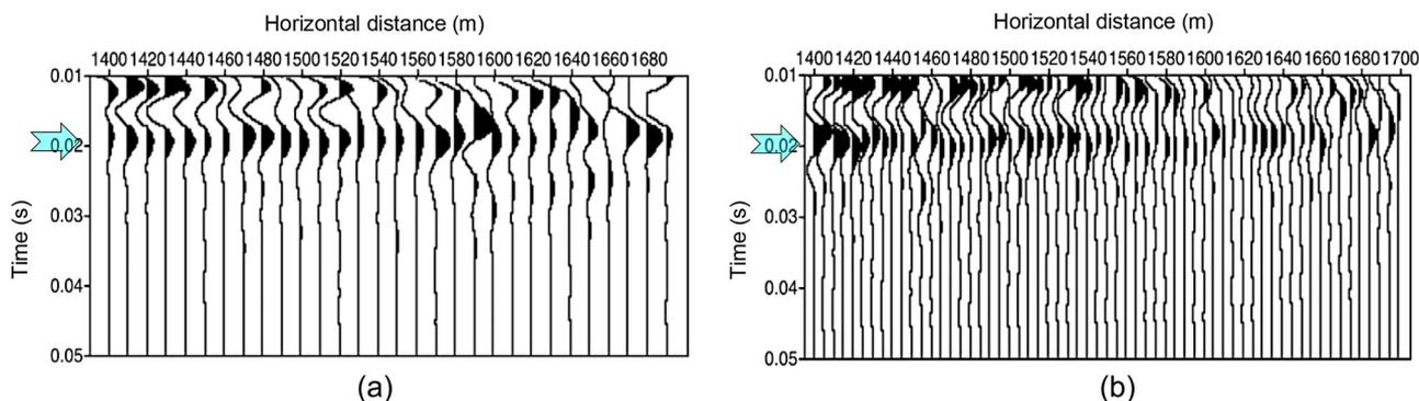
**FIGURE 6** Result of seismic interferometry (SI) by auto-correlation (AC) applied to field data: (a) to turn active sources into virtual receivers and (b) to turn the receivers into virtual sources. The cyan arrows indicate the retrieved ghost reflection.
