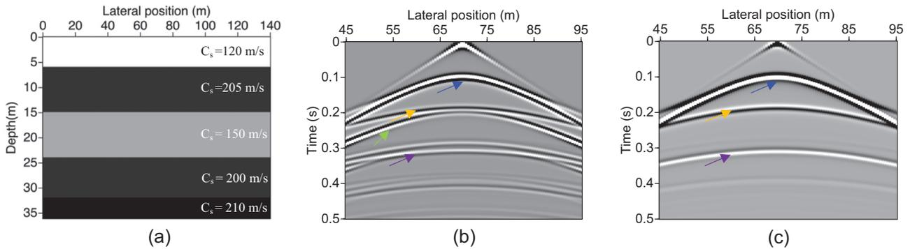
**FIGURE 2** (a) Shear-wave velocity ( $C_S$ ) model for the base survey; (b) directly modelled reflection response for an active source at (70,0) m, (c) the same as (b) but when the model has an absorbing boundary condition at the surface. The colour-coded arrows indicate the events described in Table 1.
