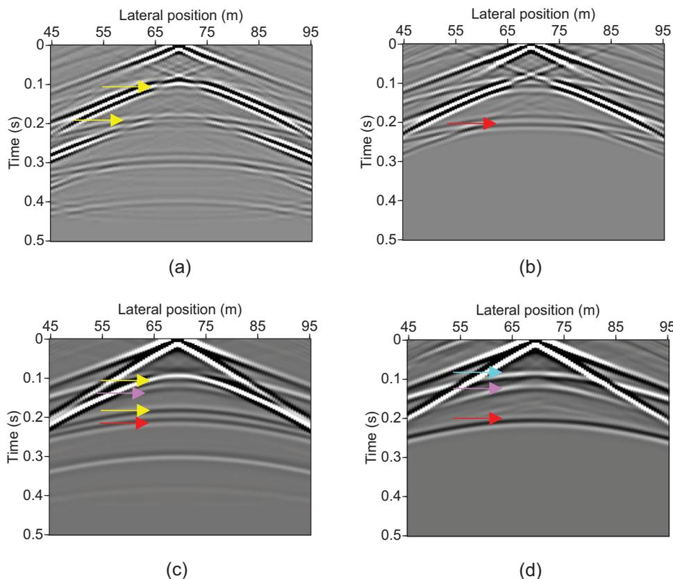
**FIGURE B1** (a) Retrieved results of seismic interferometry (SI) by cross-correlation (CC) for a virtual source at (70, 0) m (b) as in (a), but for active-source gathers which are muted before the reflection from the bottom of the first layer and after the reflection from the bottom of the third layer, (c and d) same as (a and b) but when the model has an absorbing boundary condition at the surface. The colour-coded arrows indicate the events described in Table 1.
