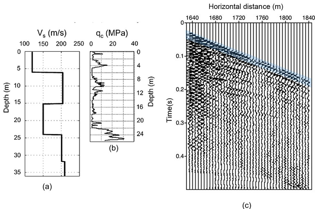
**FIGURE 5** (a) Interval velocity obtained from the root-mean-square velocity, and (b) the CPT cone-tip resistance at the same site (Ghose and Goudswaard, 2004). (c) Example of an active-source shot gather, where the source is located at 1635 m (the blue highlighted region shows the extracted reflection arrivals used for SI by AC).
