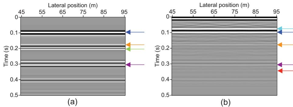
**FIGURE A1** (a) The zero-offset section obtained using the full active-source data for the subsurface model shown in Figure 2a, (b) the virtual zero-offset section retrieved from seismic interferometry (SI) by auto-correlation (AC) using the full active-source gathers.
