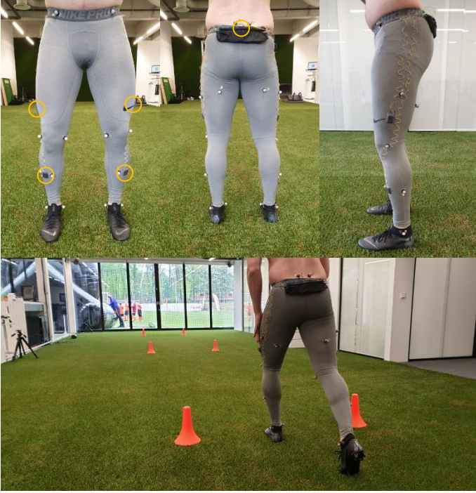
Fig. 1 The experimental test set-up used in this research study. The subject wearing the Smart Sensor Shorts (top) and the measuring volume (bottom). The locations of the five IMUs on the Smart Sensor Shorts are indicated with the orange circles (top left and top center).
