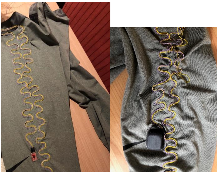
Fig. 8 The IMU attached to the tights before (left) and after the casting procedure.
