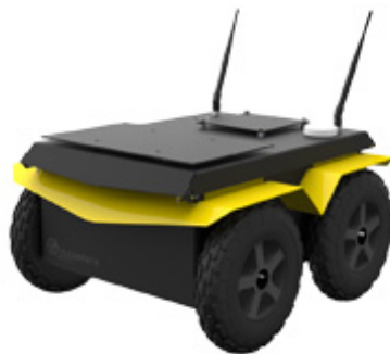
Figure 2.1: A picture of the Jackal robot: an unmanned ground vehicle using differential steering.
