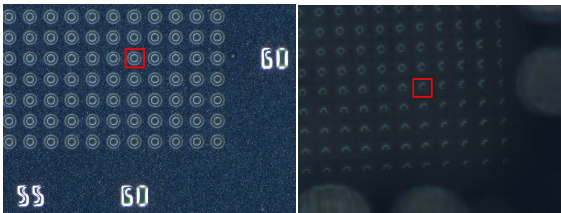
Figure 6.6: Left: microscope image of the upper (fifth) tynode. Right: fourth tynode, image obtained by looking trough the fifth tynode. The 5th diagonal dome is shown with a red square, for these domes the position was determined.
