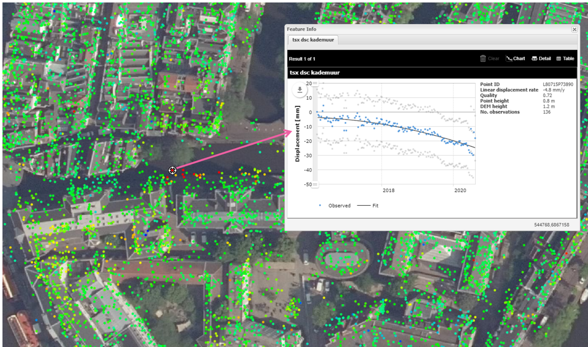
Figure 1.1: Monitoring batch result of a collapsed quay wall in the city center of Amsterdam (SkyGeo, 2023). The colored points represent scatterers in Amsterdam with the color indicating the average displacement velocity. The framework plot shows the behavior of a selected point at the collapsed quay wall indicated with a marker. The blue framework dots represent the displacement estimates and the grey dots the solutions of plus and minus one ambiguity level. This point accelerates in time, exemplified by the black line fit, until the collapse on the 1st of Sep 2020.
