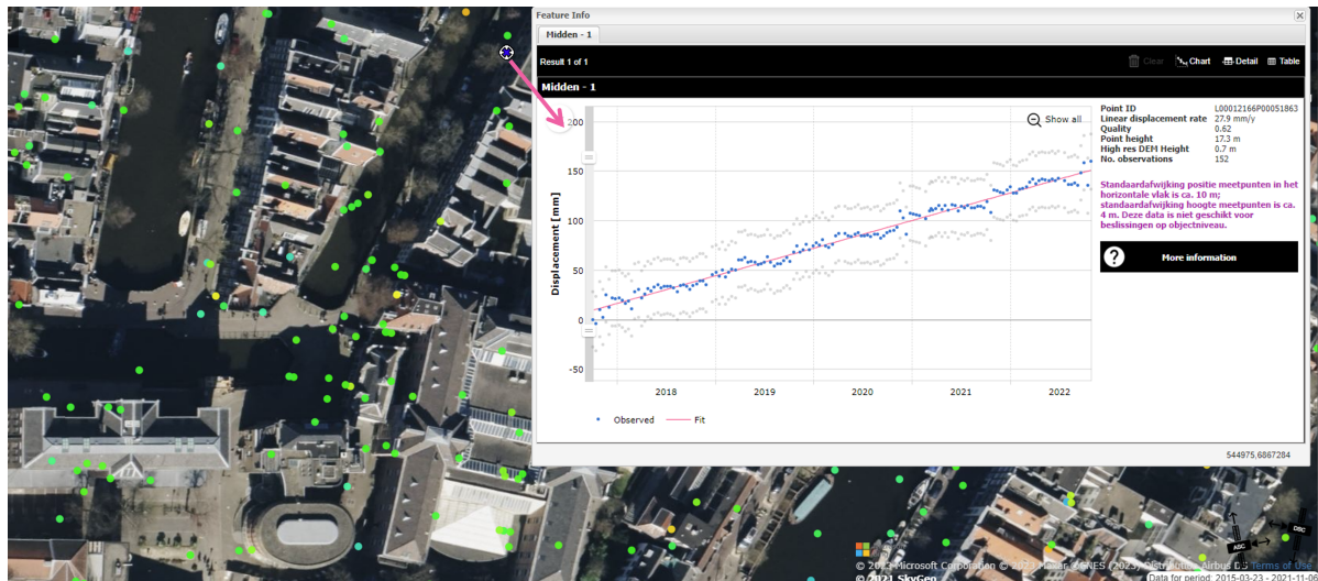
Figure 1.2: Monitoring batch result of a quay wall perpendicular to the collapsed quay wall in Fig. 1.1 the city center of Amsterdam (SkyGeo, 2023). The colored points represent scatterers in Amsterdam with the color indicating the average displacement velocity. The framework contains a plot showing the behavior of a selected point at a wall indicated with a marker. The blue dots in the framework represent the displacement estimates and the grey dots the solutions of plus and minus one ambiguity level. This point shows a strong uplift, though the behavior is questionable to say the least as following a different solution (grey dots) seems plausible as well.
