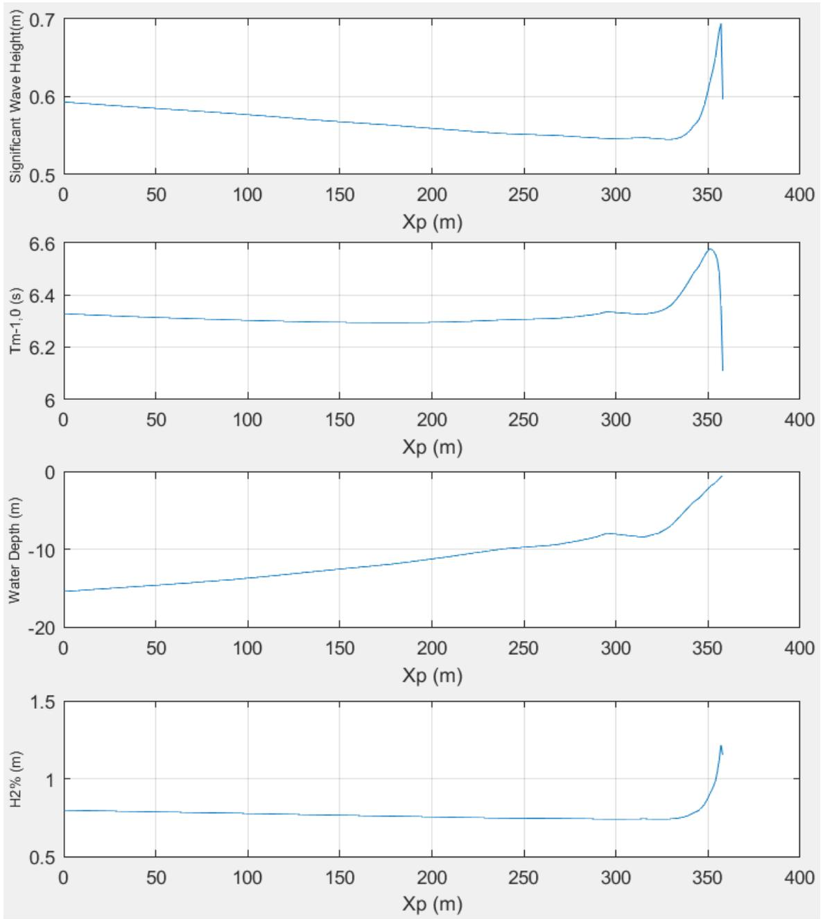
Figure 121: Cross-shore progress of several variables for mild conditions at the breakwater
