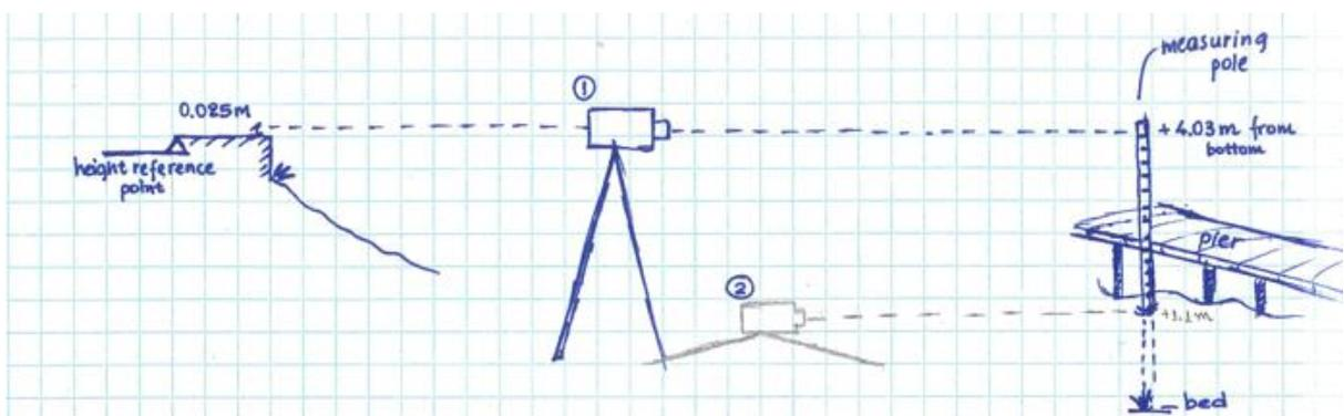
Figure 19: Mean sea level compared with reference level
