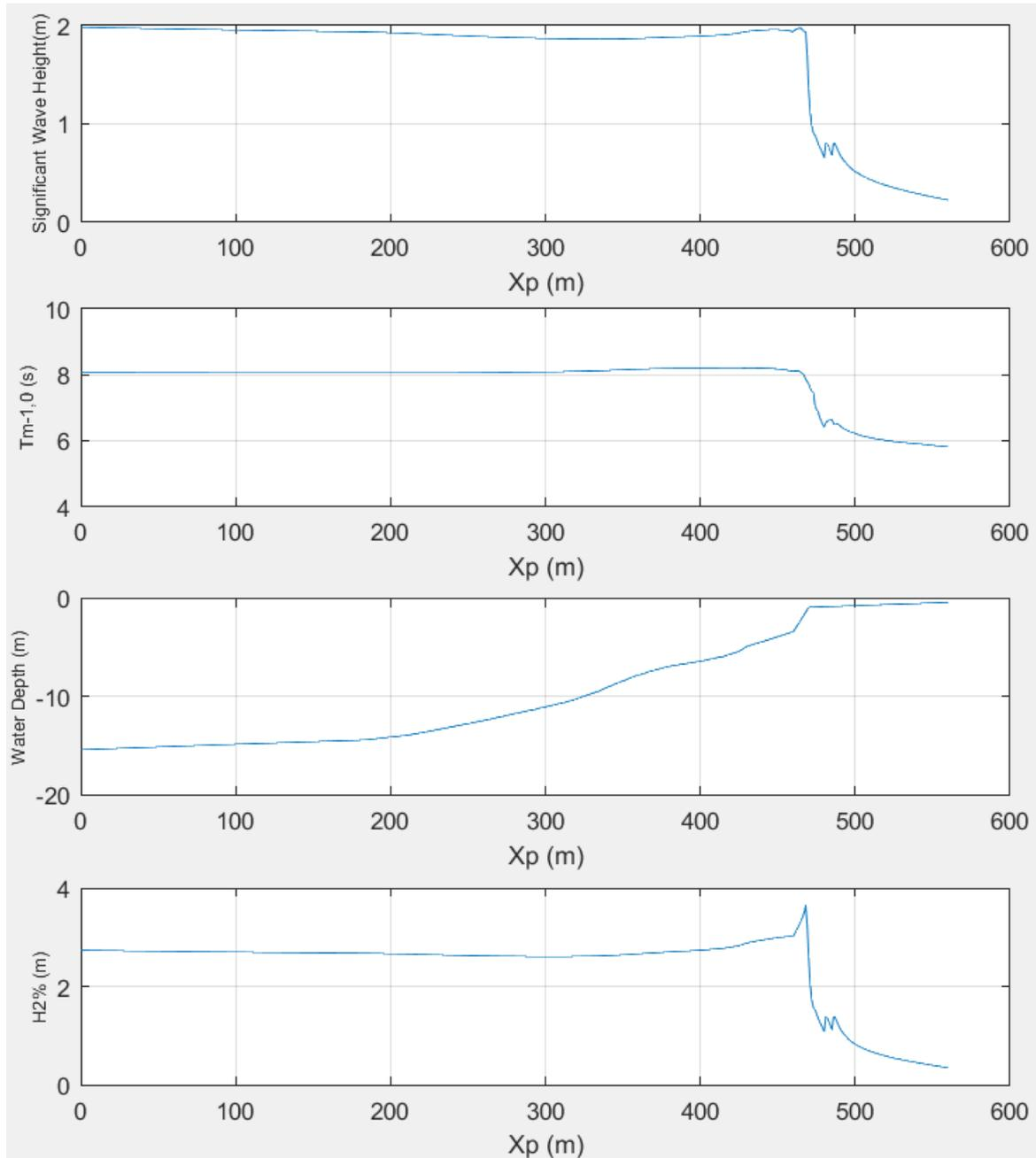
Figure 115: Cross-shore progress of several variables for severe conditions at the jetty
