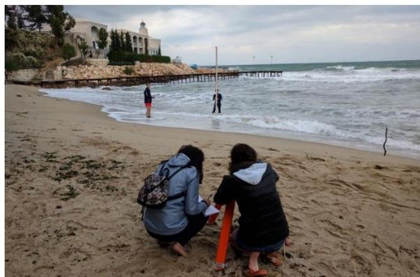
Figure 10: North beach – measuring height differences with levelling instrument and level staff
