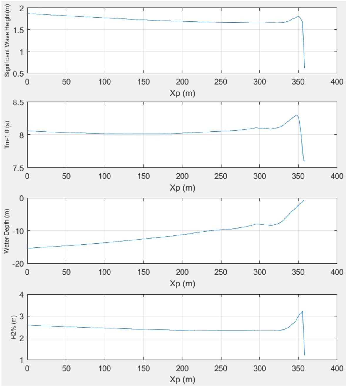
Figure 117: Cross-shore progress of several variables for severe conditions at the breakwater
