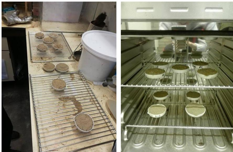
Figure 30: Samples after being dried for 24 hours
