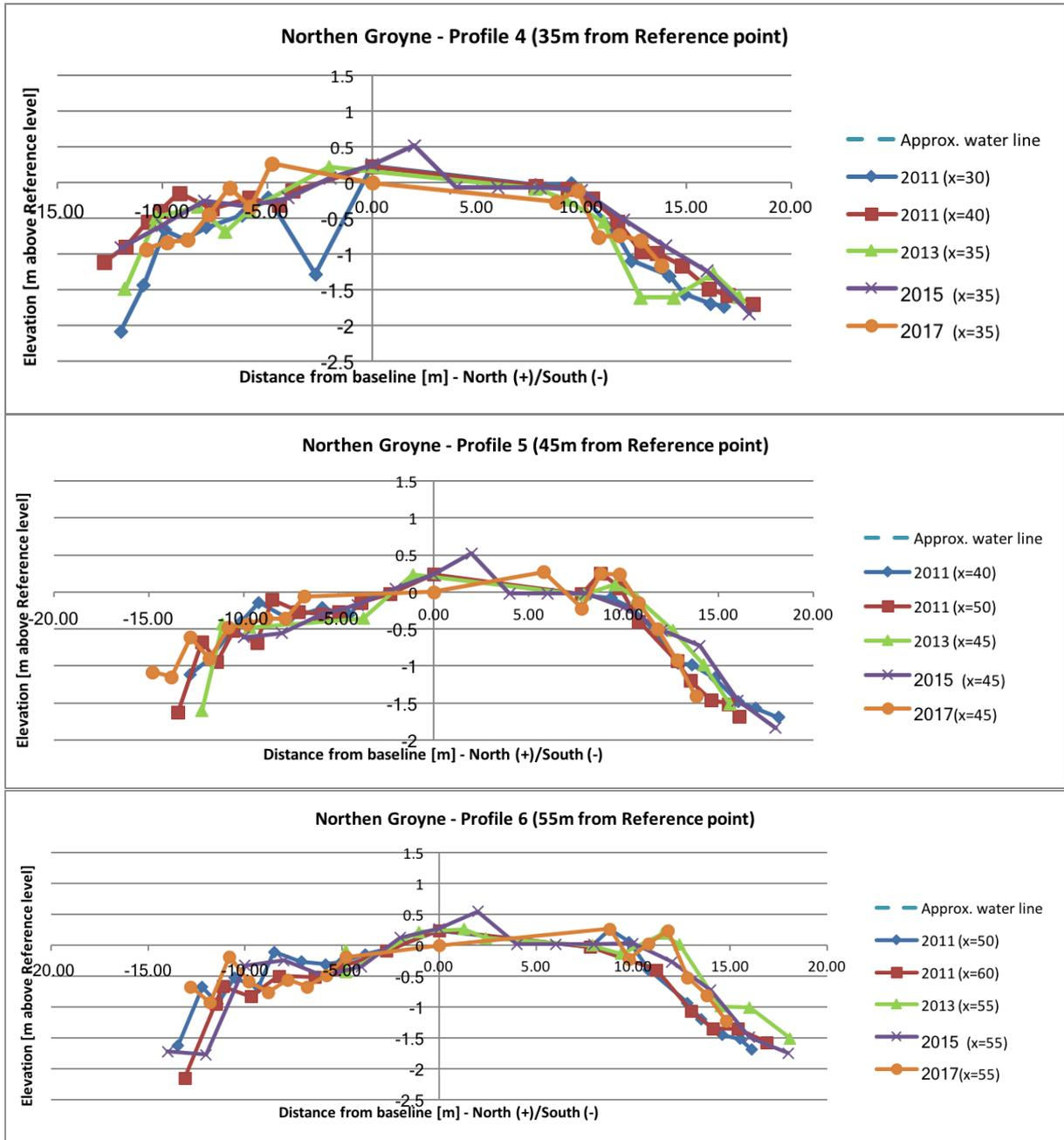
Figure 75: Measured groyne profiles of 2017 and earlier
