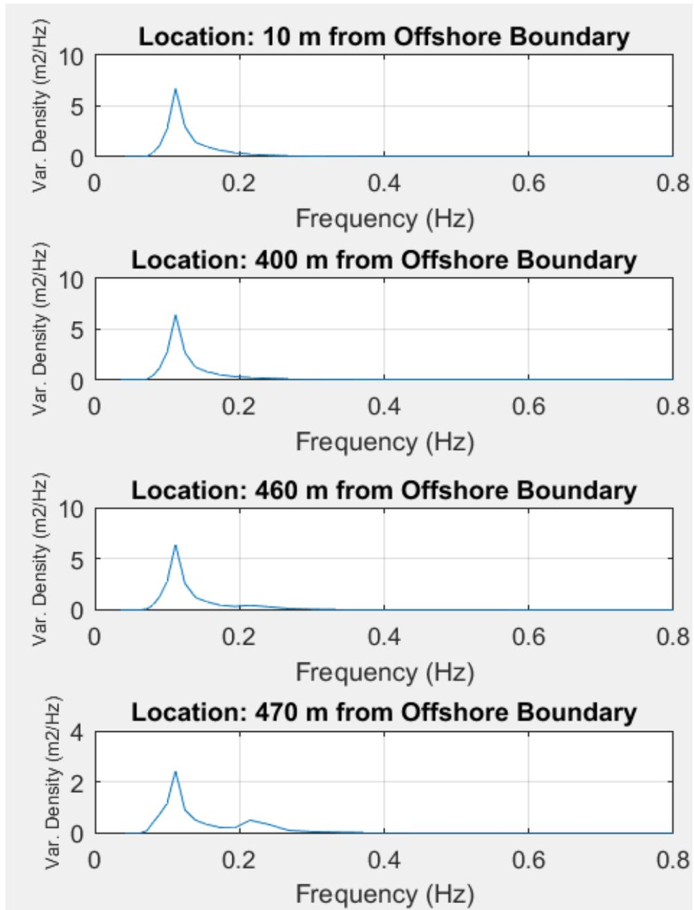
Figure 116: Energy spectra at several locations cross-shore from the jetty for severe conditions
