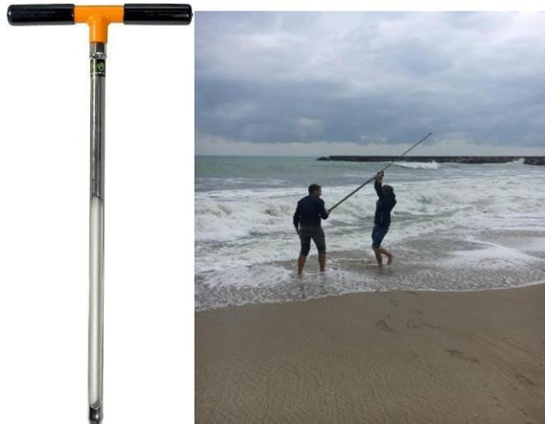
Figure 25: Tubular soil sampler (right), sampling moment (left)
