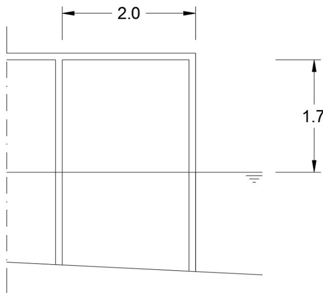
Figure 37: Jetty tip and position with respect to MSL
