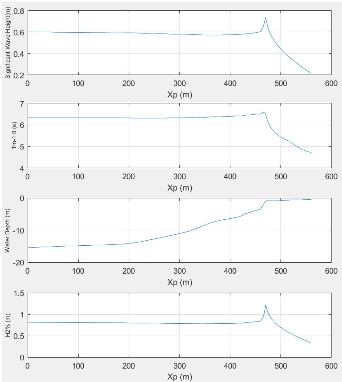
Figure 119: Cross-shore progress of several variables for mild conditions at the jetty
