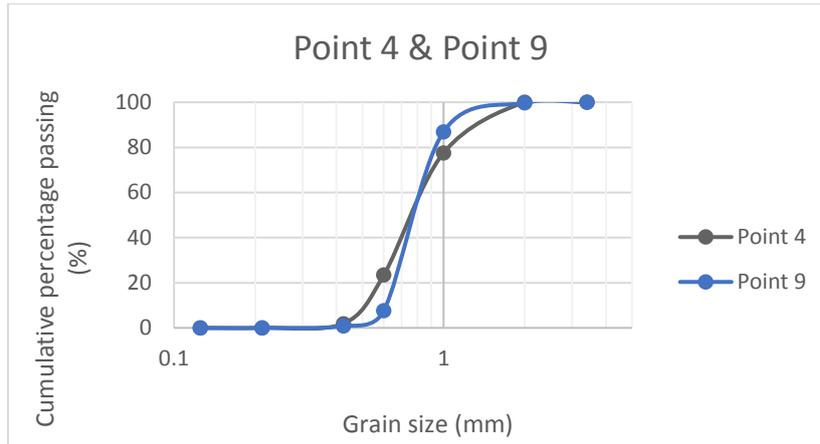
Figure 67: Sieve curves of points on the same line perpendicular to the coast – beach and offshore
