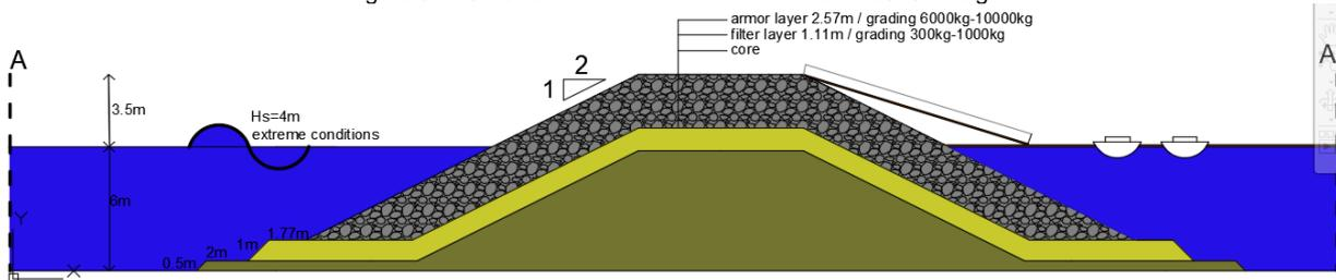
Figure 95: Cross-section A-A new design (2017)
