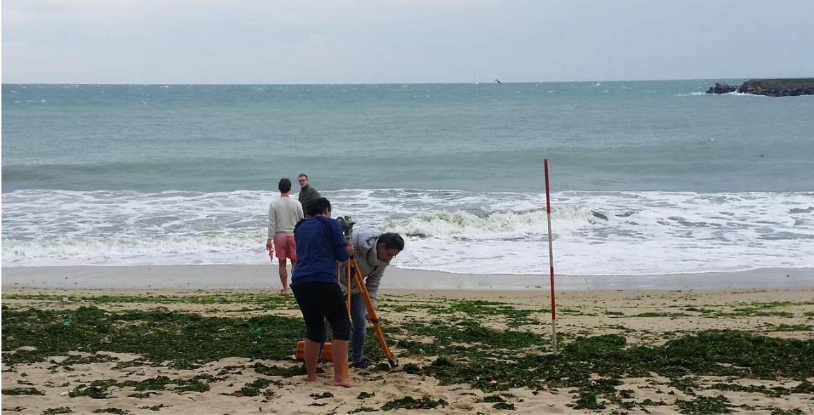
Figure 12: south beach - Levelling the theodolite by adjusting the tripod legs and using the bulls-eye level
