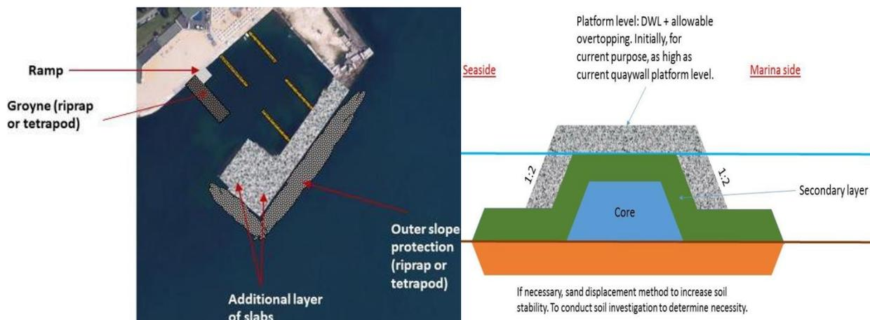
Figure 4: Sketch of the proposed layout for the marina (left), cross-section of the proposed groyne (right).
