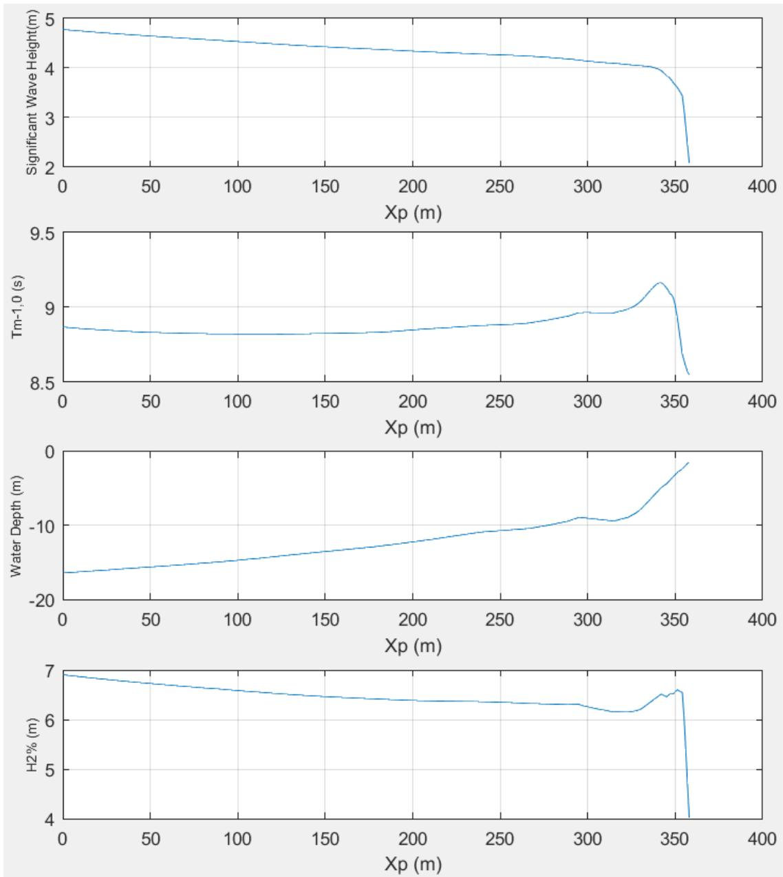
Figure 123: Cross-shore progress of several variables for extreme conditions at the breakwater
