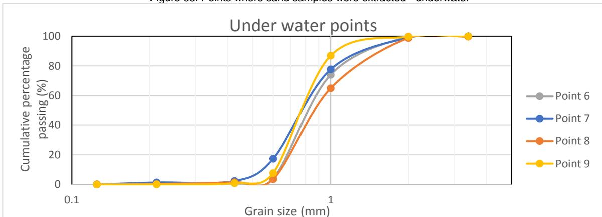
Figure 69: Sieve curves – underwater points
