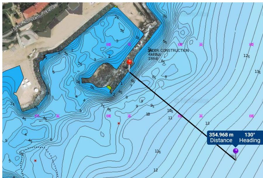
Figure 40: Cross-shore distance for the location of the breakwater
