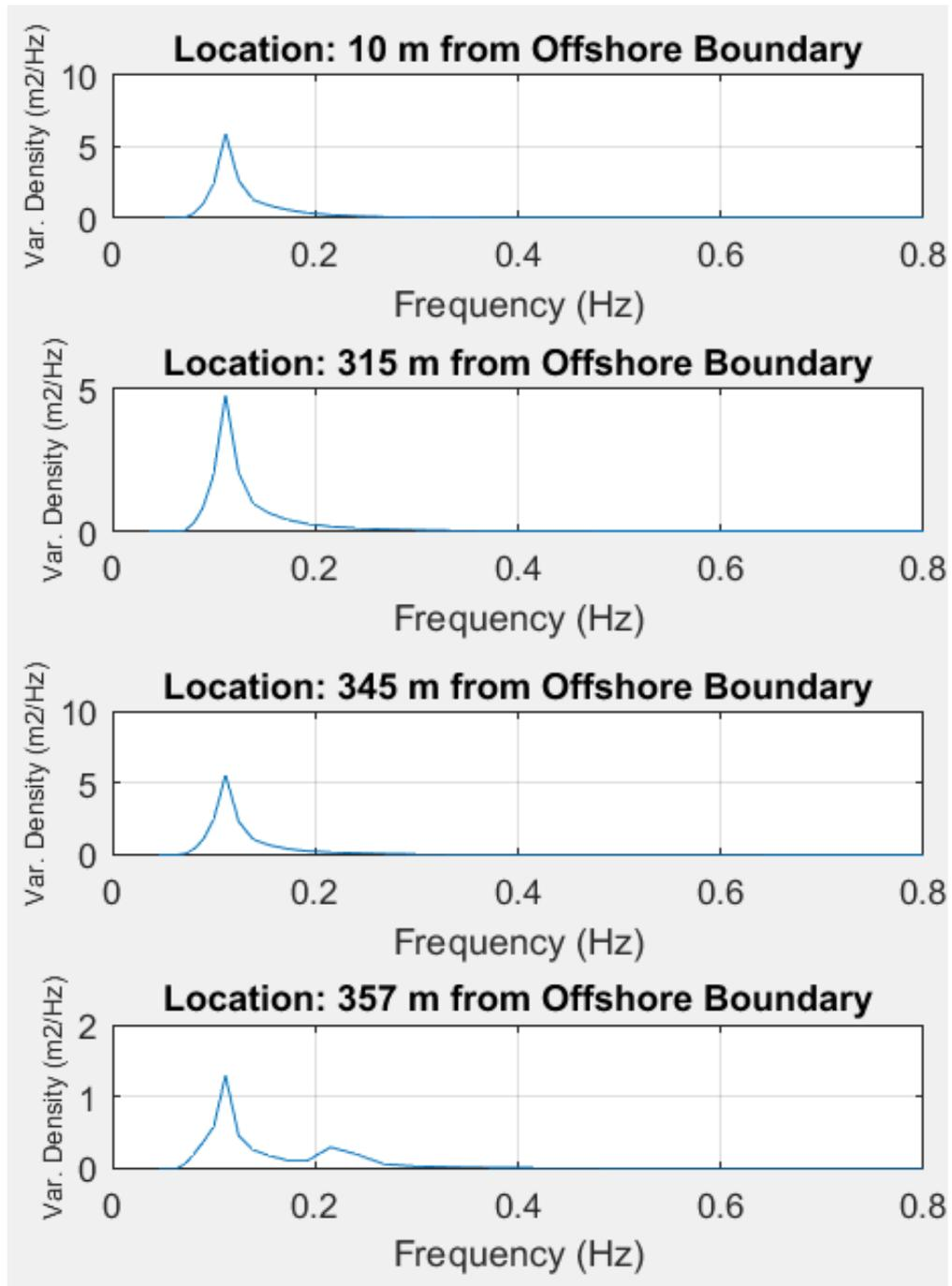
Figure 118: Energy spectra at several locations cross-shore from the breakwater for severe conditions
