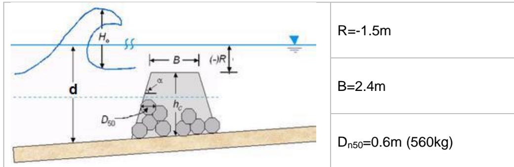
Table 1: Proposed dimensions for submerged breakwater in the North beach
