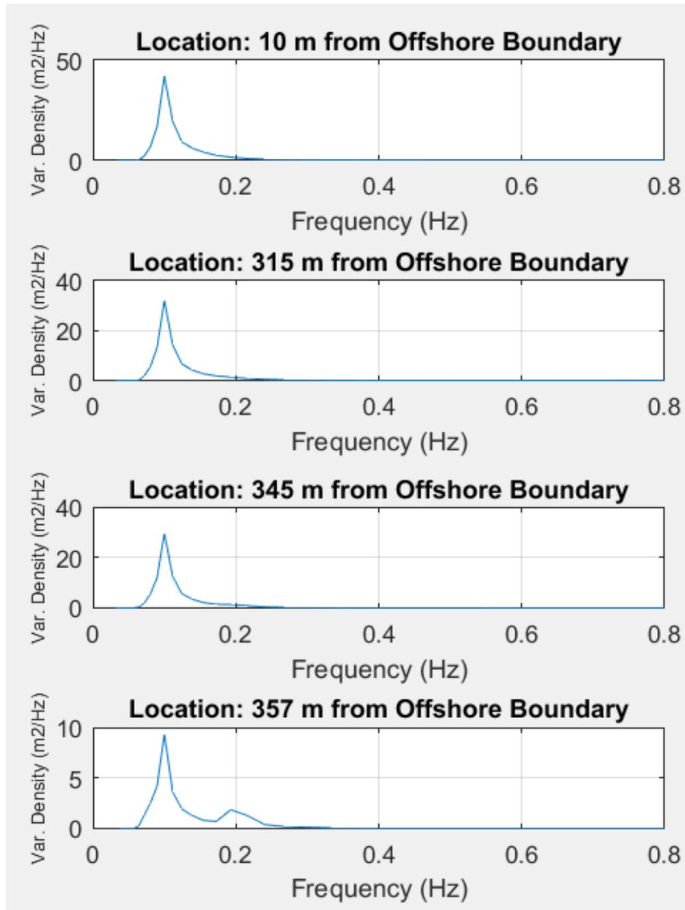
Figure 124: Energy spectra at several locations cross-shore from the breakwater for extreme conditions
