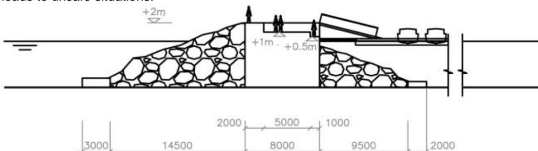
Figure 94: Cross section A-A of the breakwater in 2016 Design
