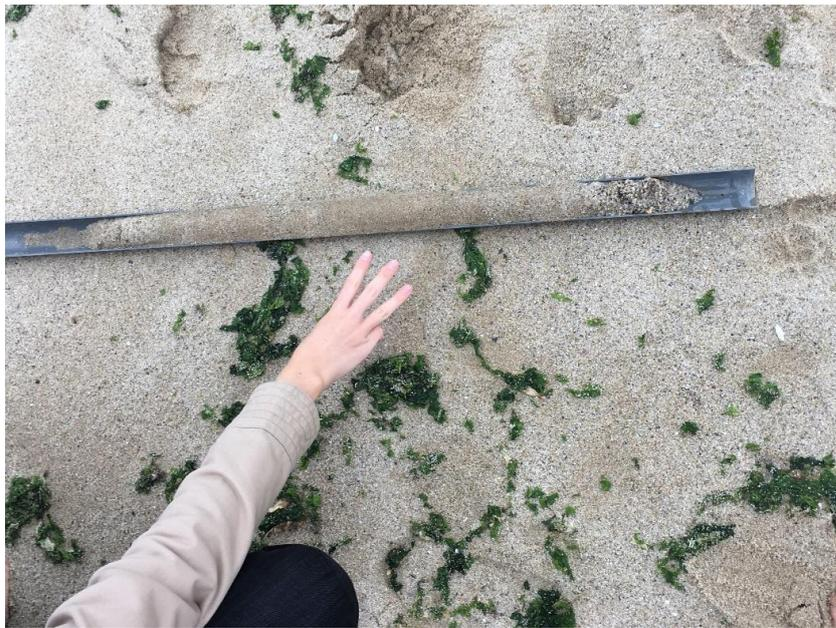
Figure 28: Sample taken with tubular soil sampler
