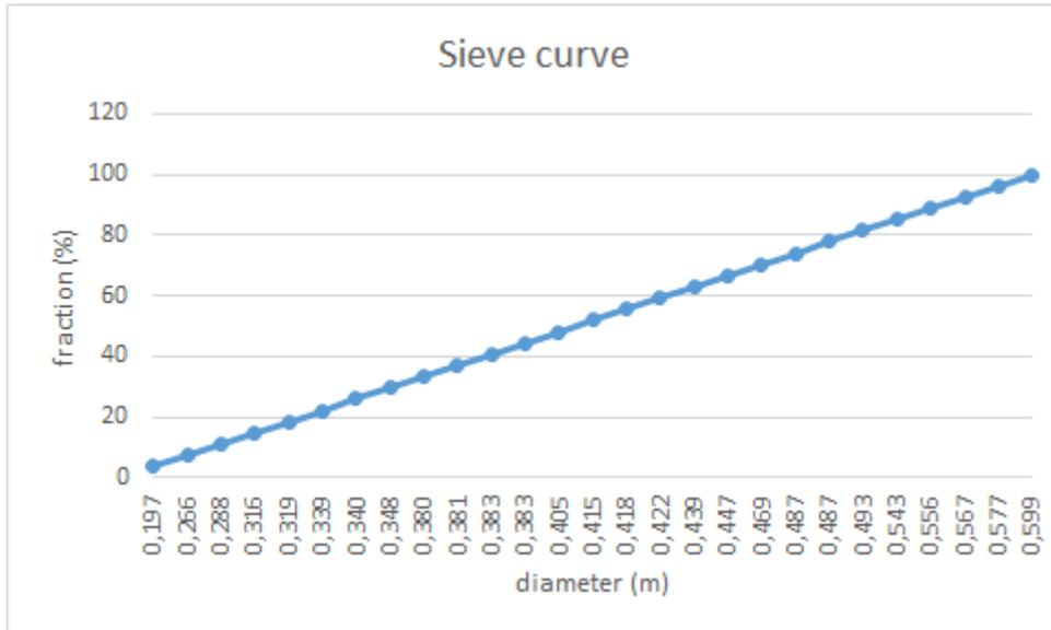
Figure 83: Sieve curve of rock samples
