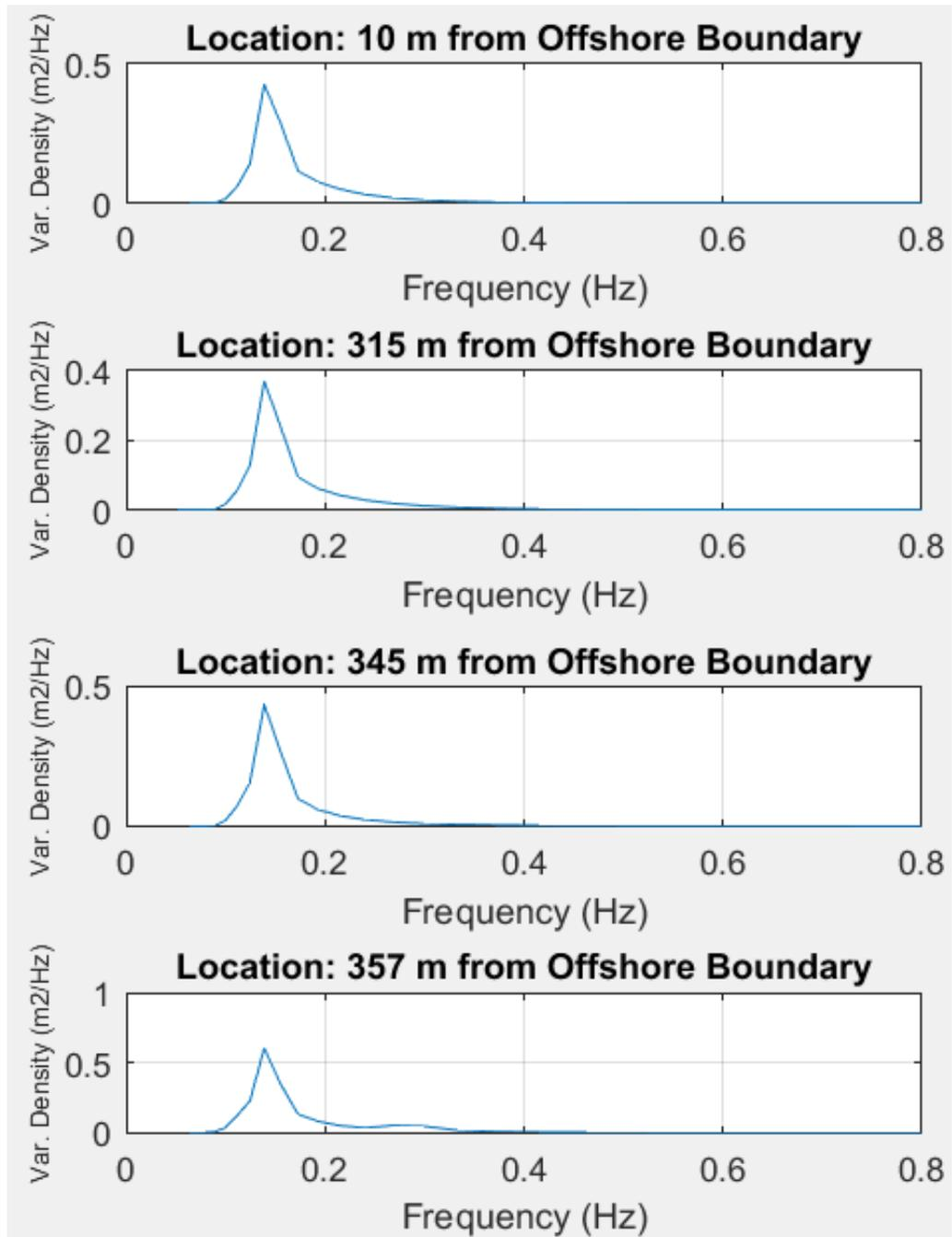
Figure 122: Energy spectra at several locations cross-shore from the breakwater for mild conditions
