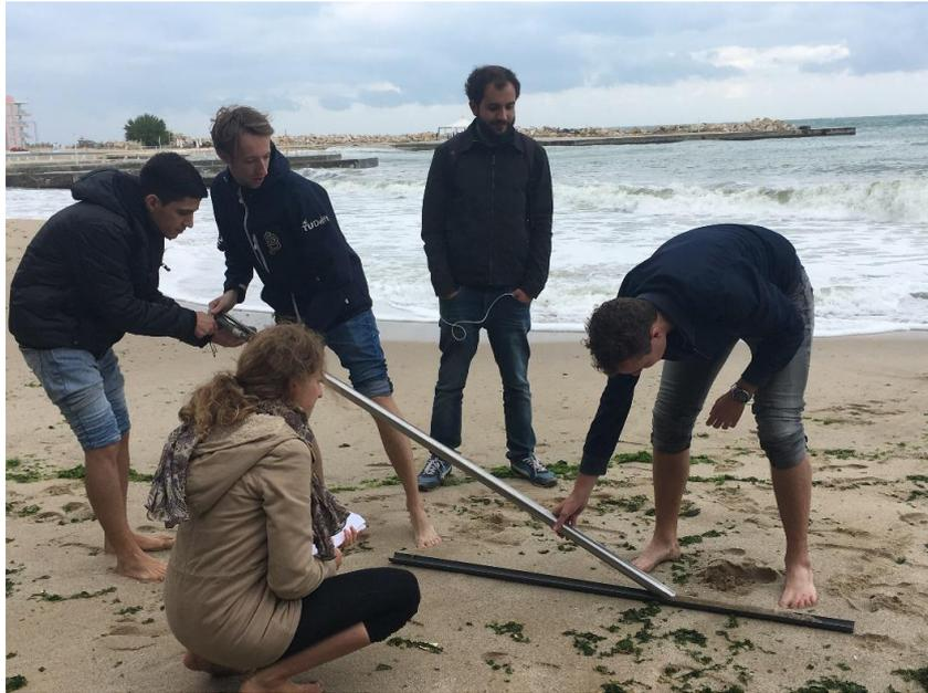
Figure 27: Procedure of extracting the soil of the tubular soil sampler
