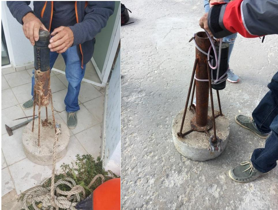
Figure 41: Wave logger 1 (left side) and wave logger 2 (right side).
