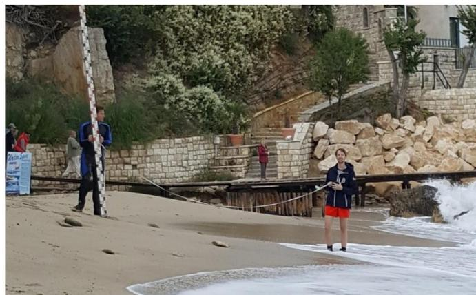
Figure 11: North beach – determining the measuring points with a tapeline
