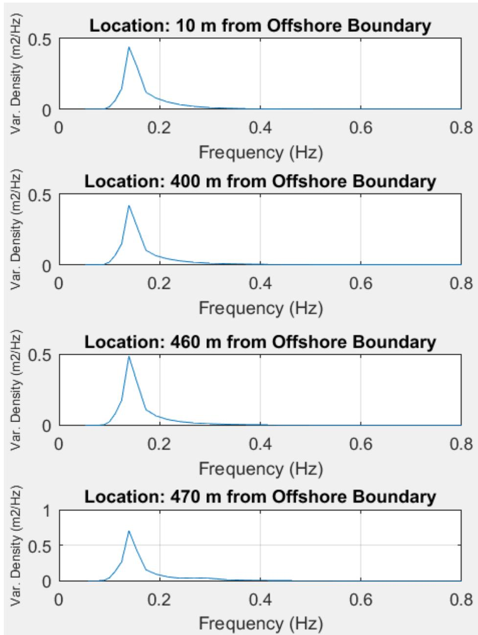
Figure 120: Energy spectra at several locations cross-shore from the jetty for mild conditions
