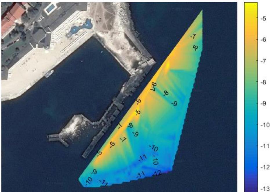
Figure 74: Bathymetry in front of the breakwater
