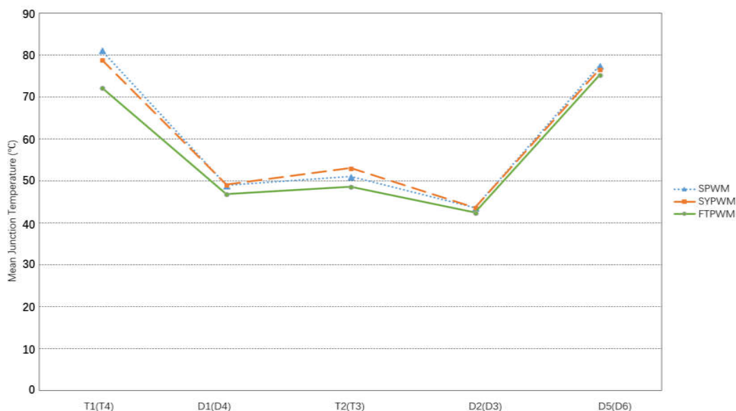
Figure 4. 23 Mean Junction Temperature Distribution at Grid Side (with 3 Modulations)
