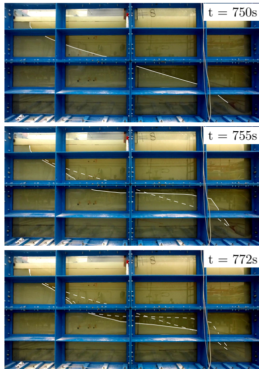
Figure 3.7: A Liquefaction failure observed during experiment 8.
