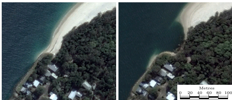
Figure 1.4: Before and after a breach failure at Amity Point. Satellite images at 2-8-2014 (left), and 18-8-2014. Taken from Google Earth.
