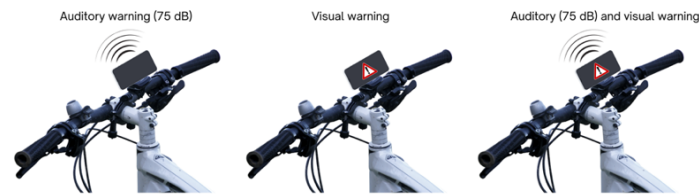
Figure 2: The auditory, visual, and visual-auditory warning system features of CycleSafe
