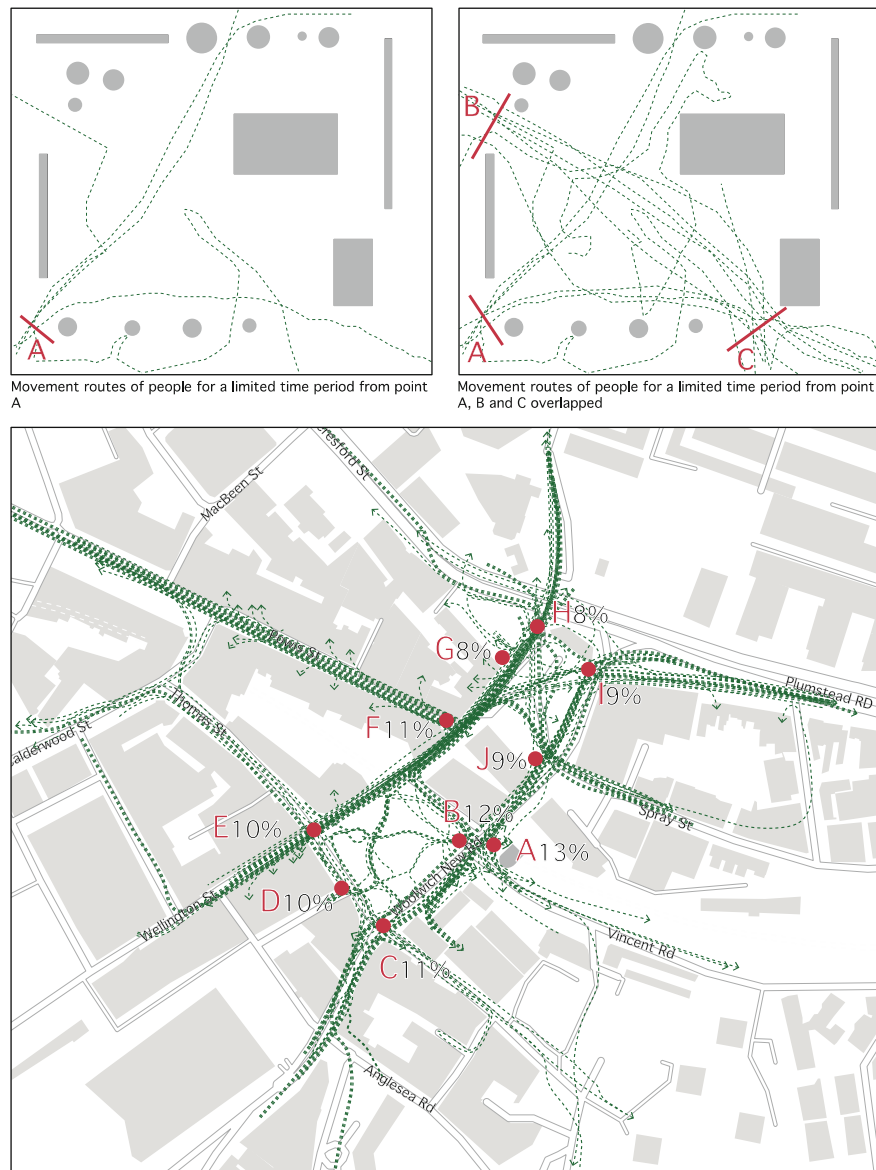
Fig. 5.8 Top: Pedestrian routes from starting point A (left) and the overlay of all registrations of starting points A, B, and C (right). Below: Overlay of all registrations of one day in Woolwich Squares in London visualised using GIS (image below – original: Space Syntax Ltd. London 2008; redrawn by authors)
