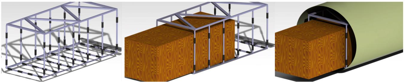
Figure 13.18: Rail system for the cargo drop system
