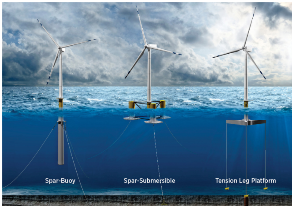
Figure 1.6: Offshore wind floating foundation concepts [6]
