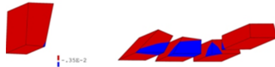
Figure 16. Concrete strains elements below the -3.5‰
