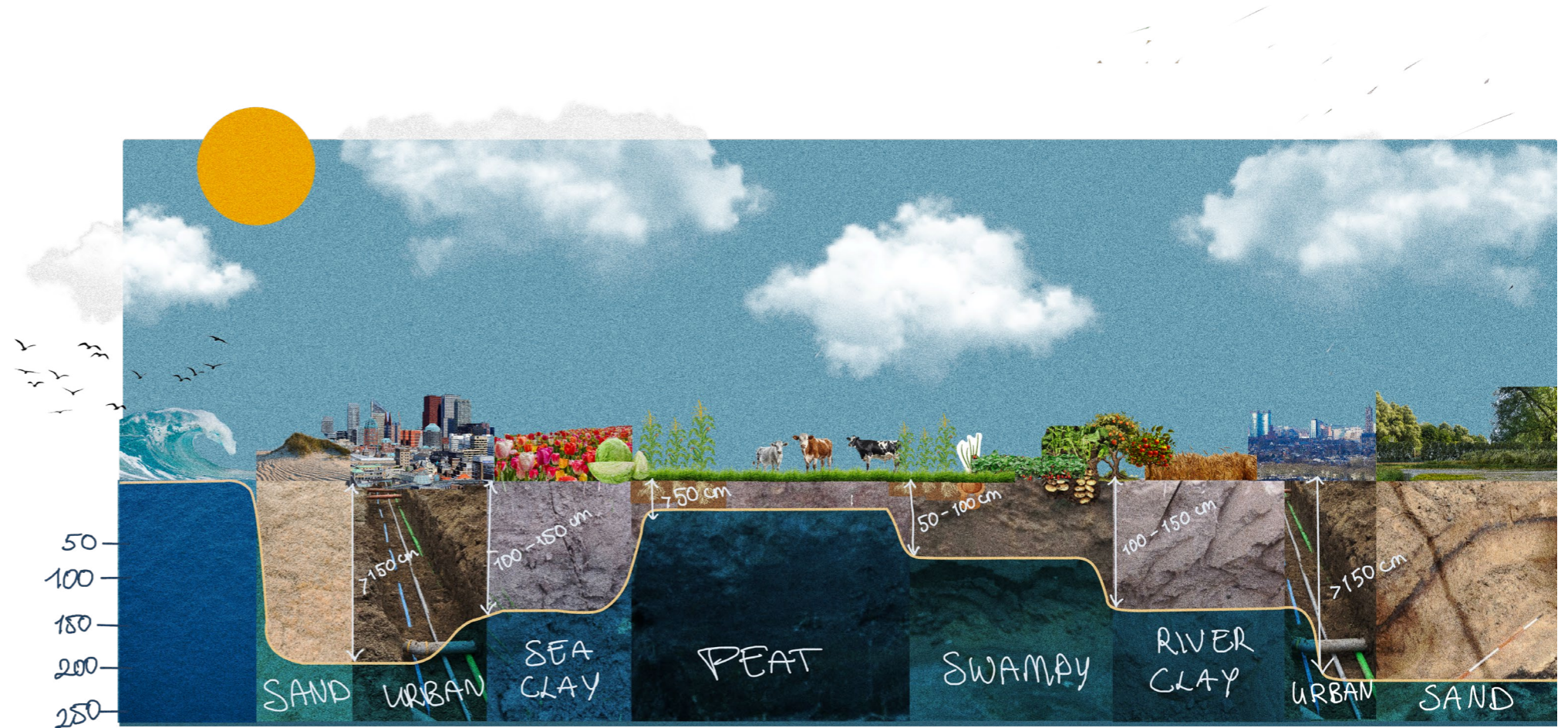
Figure 3.18: The soiltypes between The Hague and Utrecht with their characteristic watertables and vegetations.
