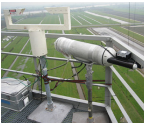
Figure 3.1: The FSSP mounted at 60-m level of the CESAR tower.
