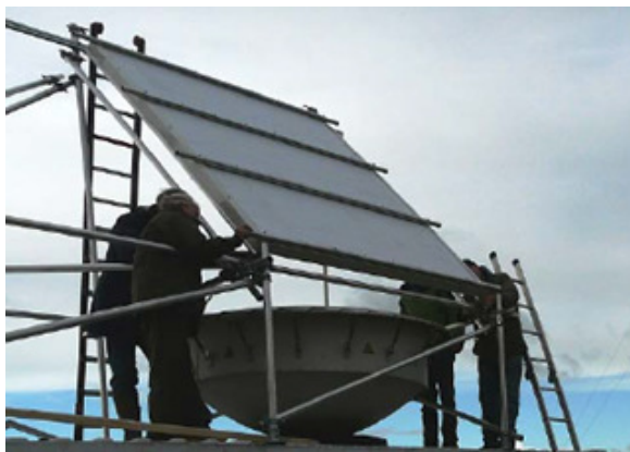
Figure 3.3: The 35 GHz cloud radar at CESAR is being prepared for the “fog mode”.
