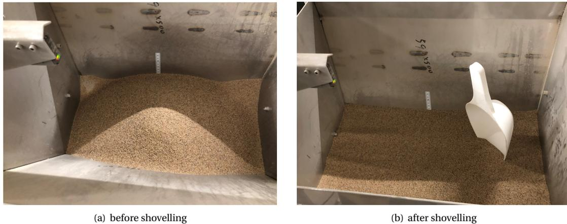
Figure 2.3: Flatness comparison of sand stored in the hopper
