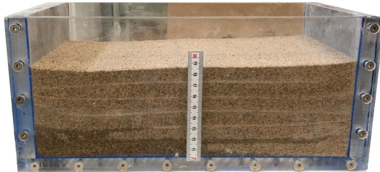
Figure 3.21: The capillary barrier effect of a pluviated specimen
