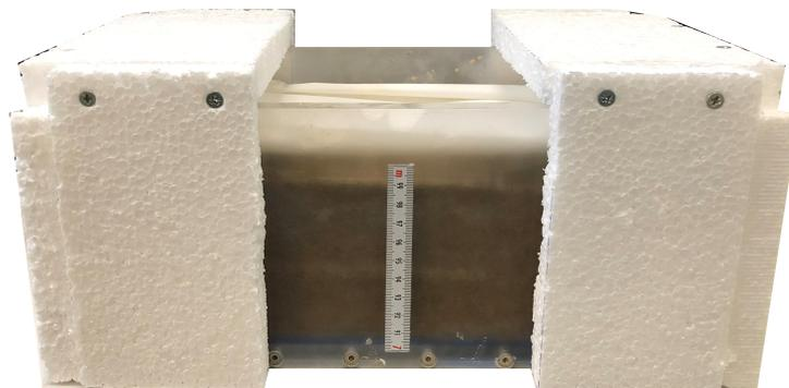
Figure 1.5: The frozen saturated specimen with controllable upheaval by using foam covers
