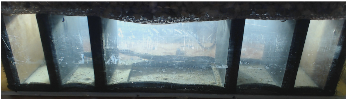
(a) A snapshot of the bottom cells inclusive initial infall before erosion was detected.
