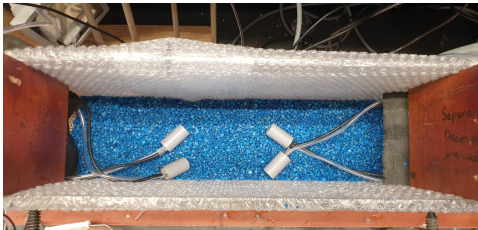
(e) Placement of half the filter layer.
