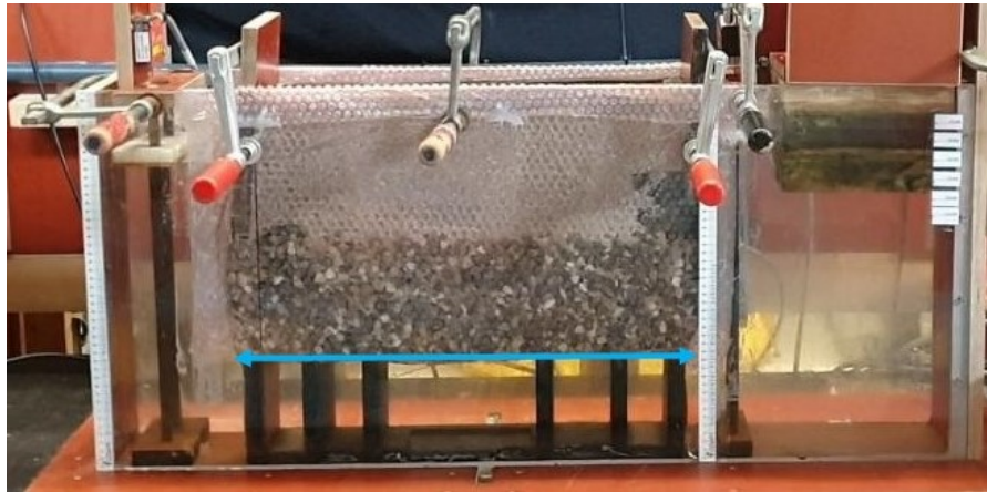
Figure 5.10: Location where water could bypass the granular filter layer.
