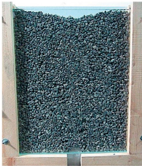
(a) Trapdoor Test Box With Gravel.
