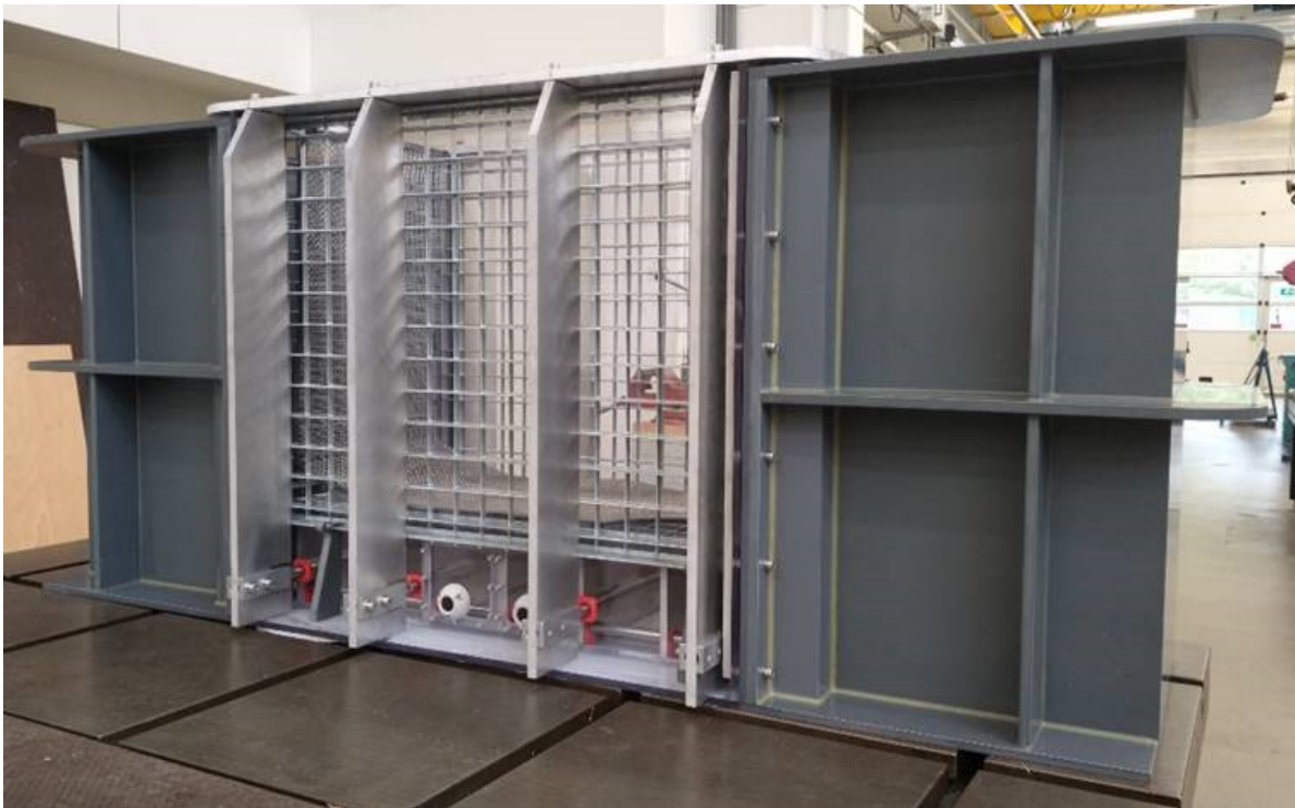
Figure 7.3: The new physical model for superimposed load and inclined filter tests.
