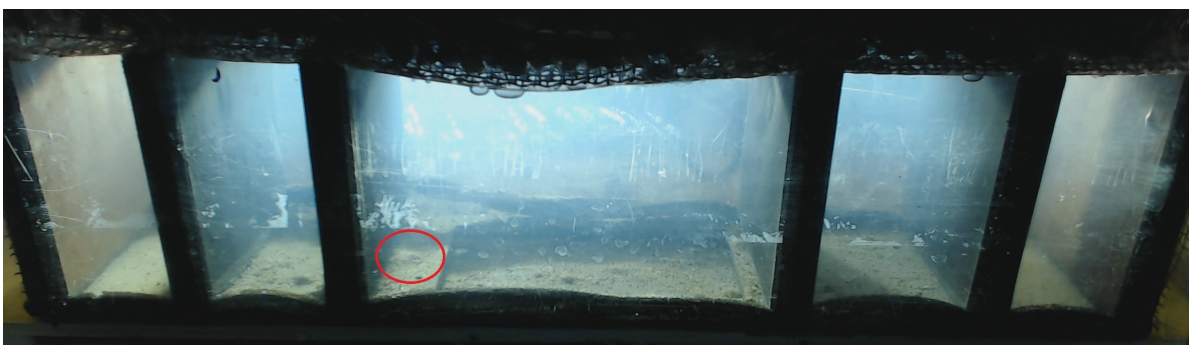
(b) A snapshot of the bottom cells in which erosion was detected, highlighted in the red circle.
