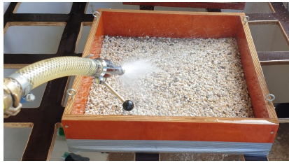
(a) Cleaning the filter layer.
