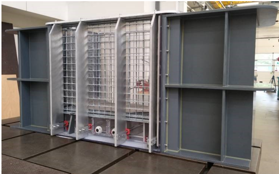
Figure 6.1: The new physical model for superimposed load and inclined filter tests.
