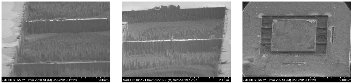
Figure 5.5: Pictures taken by a SEM show that the non-etched surface of diamond stays clean, whereas the etched surface consists of thousands of nanopillars. The sidewalls are steep, but not smooth.
