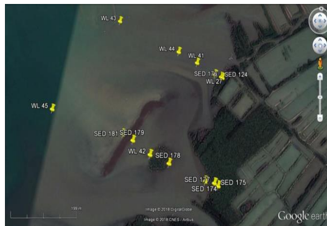
Figure 3.10(a) Locations of the wave loggers in the project area (source: Google Earth)
