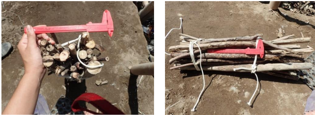
Figure 3.5 Sample of the brushwood material used in Demak (Gijón Mancheño, 2017)
