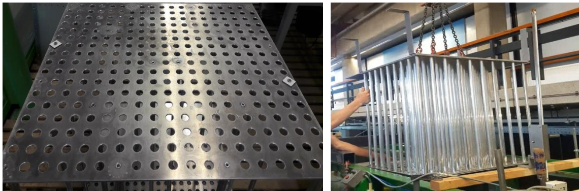
Figure 3.7 (a) Top view of design of the grid for both ends of the cylinders (b) Actual grid (c) Grids on both ends of the cylinders (in lifted position)
