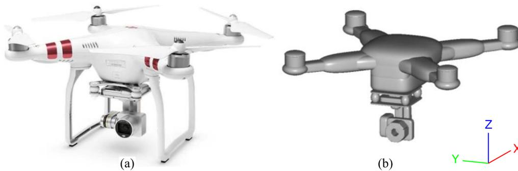
**Figure 1. UAS model for impact modelling: (a) a real-world system and (b) DJI Phantom III Standard multibody system model developed in MADYMO by the author.<sup>9</sup> The two landing skids are neglected in the model since they are not in contact with the human head in impact cases that are investigated.**
