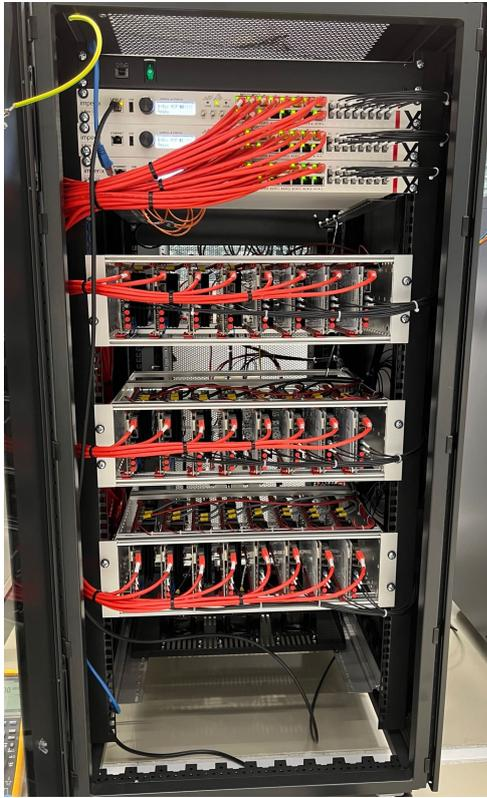
Figure D.1: Imperix MMC test bench, front view
