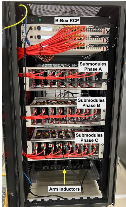
Figure 7.1: Internal configuration of the Imperix MMC.
