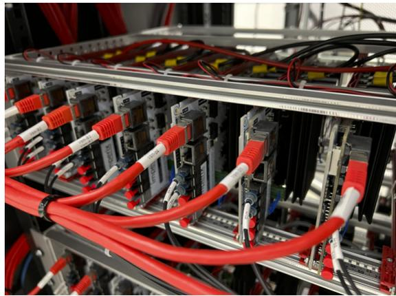
Figure D.2: Imperix MMC test bench, leg submodules
