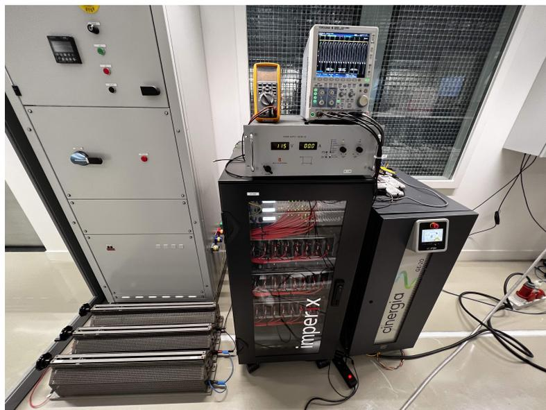
Figure D.3: Measurement setup with the Imperix MMC.
