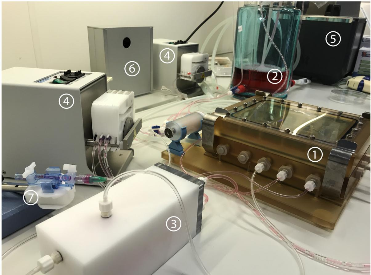
Figure 2.1: Set up of the Harvard Apparatus. Image shows: moist chamber (1), medium reservoir (2), oxygenator (3), roller pump (4), thermostatic circulator (5), mounting plate with sensors (6) and the pressure unit (7).
