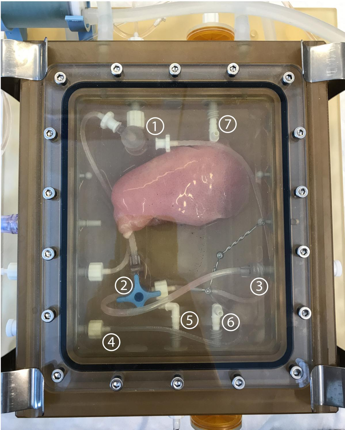
Figure 2.5: Recellularized scaffold from experiment 7 in the HA on day 13. Numbered parts are: bubble trap (1), 3-way stopcock (2), inlet port of injections (3), tube going from cannula to the pressure gauge (4), medium outlet (5), air outlet (6), air inlet (7)
